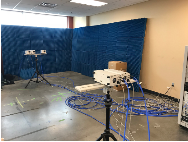
Fig. 4: CREW Monostatic radar (foreground), target and PU simulators (background). The blue phased-matched cables connect the transmit and receive heads to the main control rack
