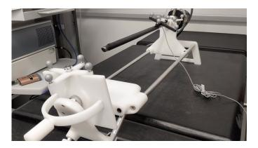
Figure 3: Completed rig assembly for calibrating the laparoscope for use in the system.
