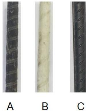
Figure 1 Photo of the reinforcing bars (A: BFRP bar; B: GFRP bar; C: steel bar)
