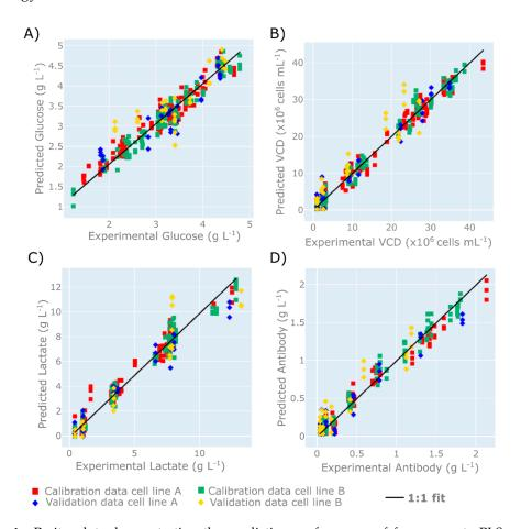
**Figure 4.** Parity plots demonstrating the prediction performance of four separate PLS models, highlighting the calibration and validation data sets of cell line A and B for (**A**) glucose concentration, (**B**) viable cell density (VCD), (**C**) lactate concentration, and (**D**) antibody concentration.
