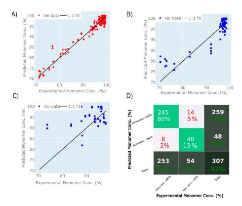
**Figure 7.** Prediction performance of the PLS model predicting the monomer purity of the fusion protein with (**A**) displaying a parity plot for validation set T1, (**B**) parity plot for calibration set P1, (**C**) parity plot for calibration set P2, and (**D**) confusion matrix that classifies the monomer purity predictions above or below 90% in comparison to the experimental monomer purity.
