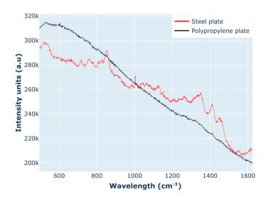
**Figure 9.** Comparison of acquisition settings of the spectra recorded by HT Raman spectroscopy microscope using polypropylene plates (in black) compared to the improved acquisition settings using stainless steel (SS) plates, a higher laser power, and higher magnification objective (in red).
