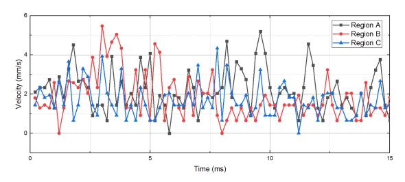
Figure 2: **Instantaneous tracer velocity measurements.** The instant speed of W tracers in region A, B and C were carefully measured by calculating the displacement of W tracers over each frame of the radiography. The max speed of the W tracers in the melt pool is  $5.5 \, \mathrm{mm \, s^{-1}}$  and the average speed in all regions is  $2 \, \mathrm{mm \, s^{-1}}$ .
