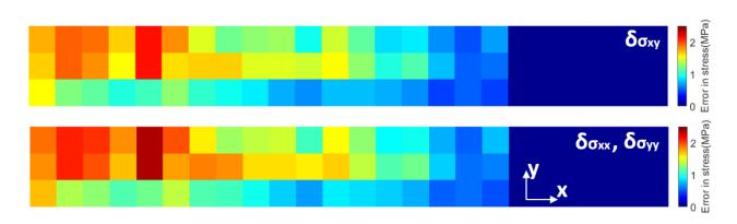
Figure 6: **Residual stress 95% confidence interval in the melt track area.** The values are calculated through error propagation from fitting error. The figure is correlated with Figure 6.
