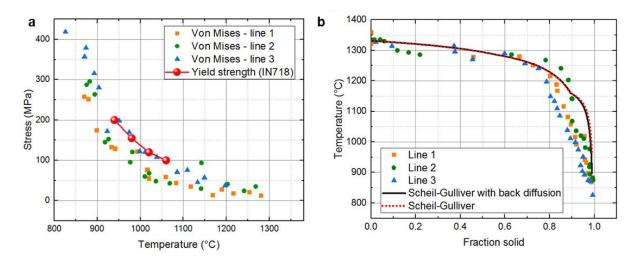
Figure 7. Cracking susceptibility of IN718 during DED-AM. (a) Von Mises stresses in the melt track region calculated against IN718 yield strength at a strain rate of 0.001 s<sup>-1</sup>. Plasticity accumulates which prevails continuously as the temperature decreases. For error calculation see Supplementary Methods(2.2.2). (b) The fraction of solids during the cooling process showing a large solidification range.
