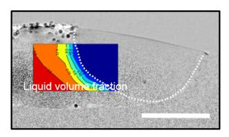
Figure 5: Liquid volume fraction calculated from diffraction patterns matches the melt pool boundary captured using X-ray radiography. Liquid volume fraction results are interpolated and show perfect gradient matching the radiography results. Scale bar  $= 1000 \ \mu m$ .
