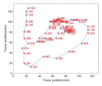
Figure 3: Instantaneous tracer velocity measurements against its instantaneous position. The instant speed of W tracers in region C were carefully measured by calculating the displacement of W tracers over each frame of the radiography. It is plotted against its instantaneous position on the radiograph, the unit is mm. The unit for the tracer velocity is  $cm s^{-1}$ .
