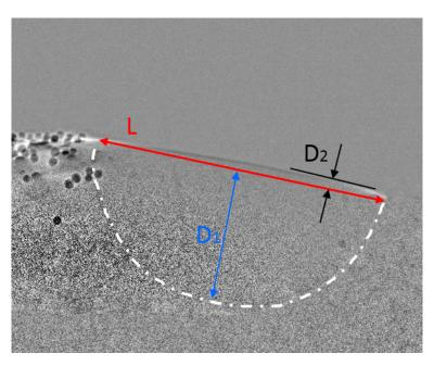
Figure 1: **Melt pool geometry measurements.** L is the melt pool length,  $D_1$  and  $D_2$  are the melt pool depth. The width of the melt pool (W) is set to be 1 mm, which is the thickness of the substrate.
