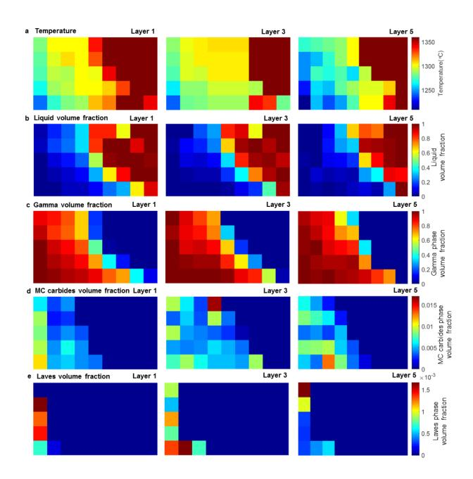
Figure 5. Melt pool mapping results derived from diffraction patterns showing (a) Temperature, (b) liquid volume fraction, (c)  $\gamma$  phase volume fraction, (d) MC carbide volume fraction, (e) laves volume fraction in multi-layer melt pool region. The liquid volume fractions mapping results match the radiography of the melt pool boundary, the results can be found in Supplementary Information.
