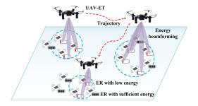
Fig. 1: Illustration of a UAV-enabled WPT with multi-beams.
