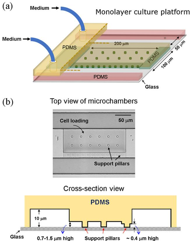
**FIG 1** (a) Microfluidic platform used for monolayer cell culture. The microfluidic part of the chip is made of polydimethylsiloxane (PDMS) elastomer, which is bonded to a glass substrate to form an enclosed device. The support pillars in the microchambers prevent potential collapse of the chambers during the bonding process. (b) Top view of a microchamber and cross-section view of the platform.
