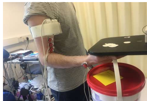
Figure II: Participant at 90 degree elbow flexion Part 2 in condition 3 and 4 as shown in Table TABLE II: Conditions for part II of the study Four unipolar electrodes are placed under
