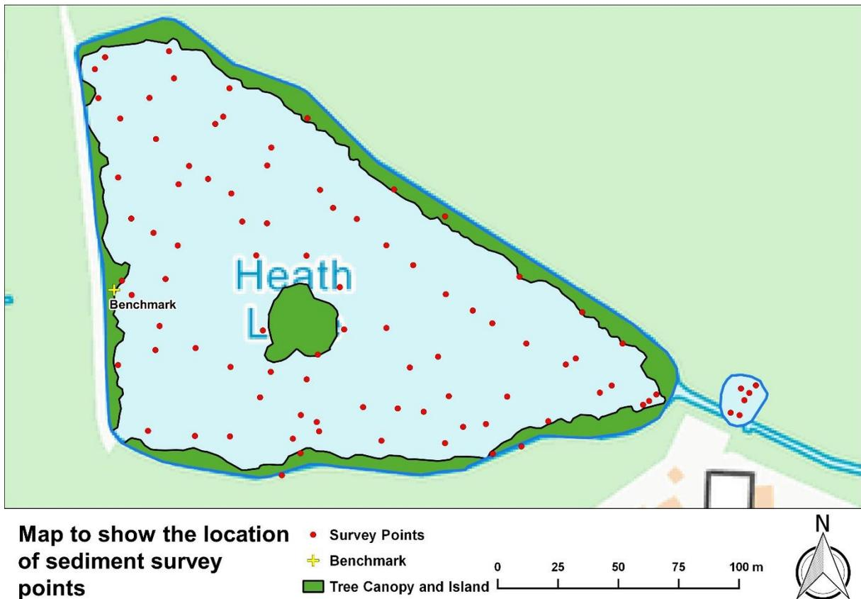
Figure 2 Map to show the survey points where water and sediment depths were measured
