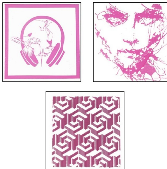
Figure 6. Three LSC samples 100 \times 100 \times 5 \text{ mm}^3 substrates patterned with ink at 15 DPI. Reproduced (adapted) with permission [51] Copyright 2020 Elsevier.
