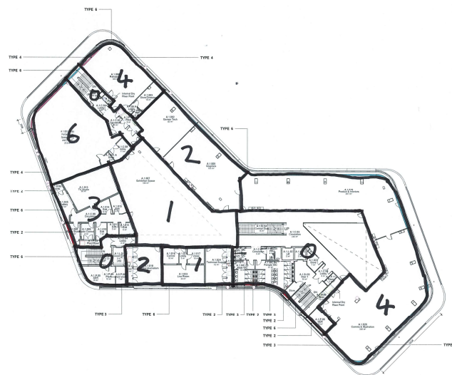
Figure 33. First floor plan showing the location of heating ventilation and air conditioning strategies zones before optimisation.
