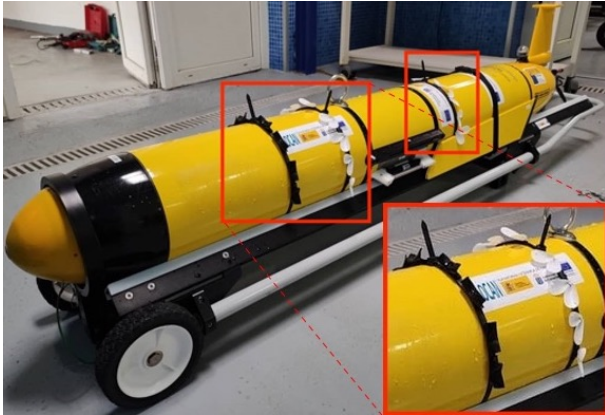
Fig. 4. Drag stimulators (highlighted by red boxes) added to the Slocum UG to simulate extreme levels of marine growth.
