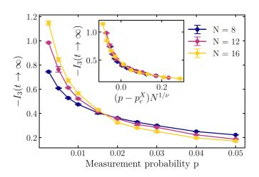
FIG. 7. Steady-state tripartite information  $I_3$  as a function of measurement probability p and system size N. The inset shows a data collapse with the fitted parameters  $p_c^{\chi} = 0.014(2)$  and  $\nu = 1.3(2)$ .
