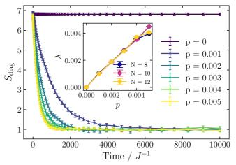
FIG. 4. Dynamics of the diagonal entropy  $S_{\text{diag}}$  using the energy eigenbasis, with Z-basis measurements and N = 12.  $S_{\text{diag}}$  is preserved by Hamiltonian evolution, so for p = 0 it remains constant in time. For p > 0, projective Z-basis measurements cause it to decay exponentially at a rate proportional to p. The inset shows the dependence of the early-time decay rate  $\lambda$  on p and N, with  $\lambda \approx p$ , independent of N.
