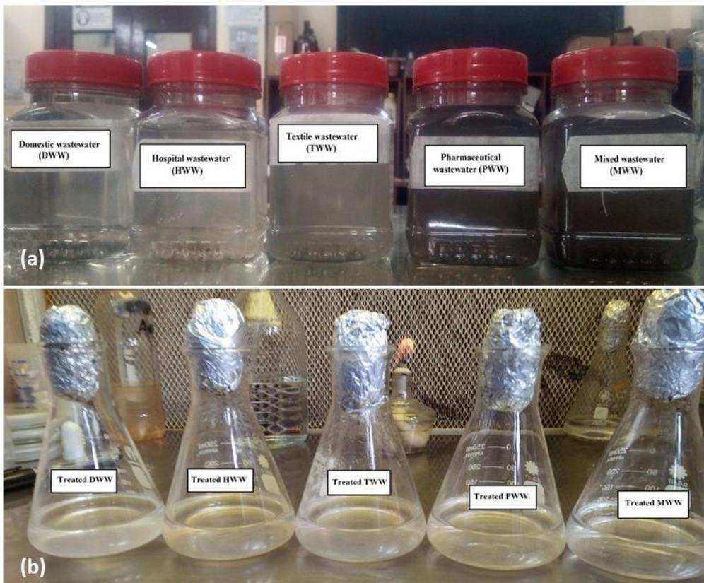
**Figure 1.** Photographic image of **a)** the untreated wastewaters (Domestic wastewater – DWW; Hospital wastewater – HWW; Textile wastewater – TWW; Pharmaceutical wastewater – PWW and Mixed wastewater – MWW) and **b)** the same wastewaters after biotreatment.
