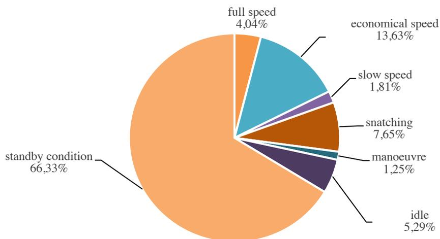
**Figure 5.** Pie chart distribution for operational condition time based generated from SHIMOS®.
