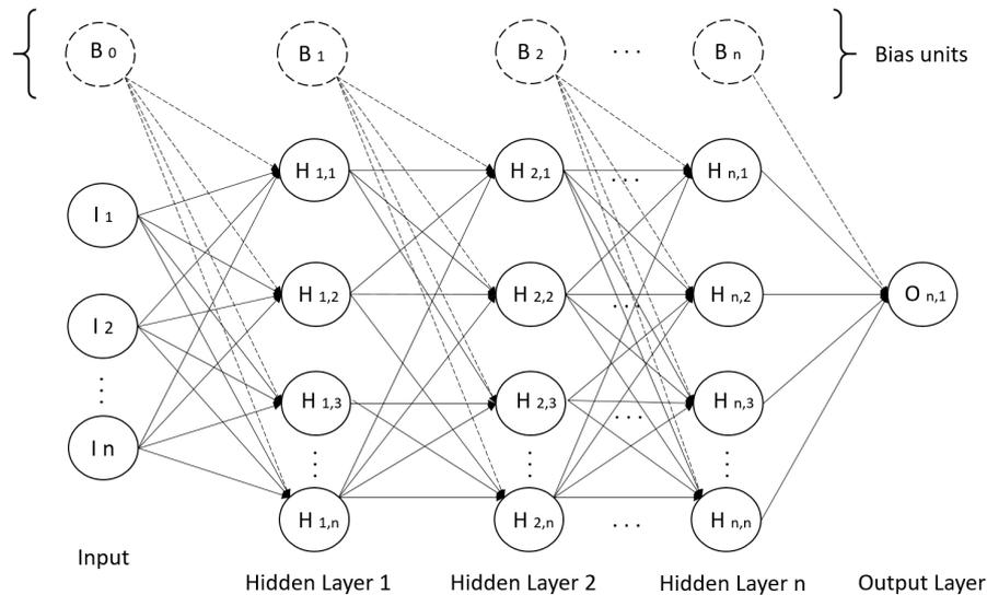
**Figure.7** Schema of Neural Network with  $n$  hidden layers and  $n$  Neuron.
