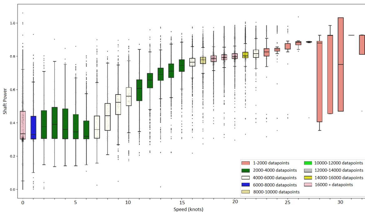
**Figure 8.** Box plot plotting at every recorded value of shaft power in scale at recorded speed.
