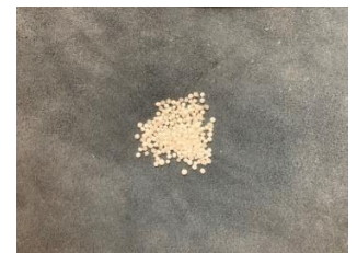
Fig 3 Paraffin pellets before coating with geopolymer slurry.
