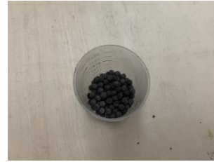
Fig 4 Paraffin pellets coated with geopolymer slurry.
