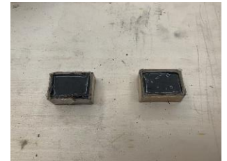
Fig 5 GPC and GPC-PCM samples at the size of 30 \times 20 \times 10 \text{ mm}
