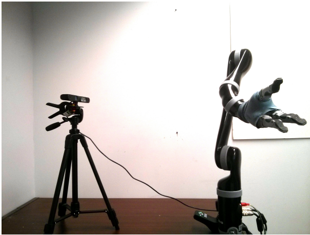
Fig. 2: Real-world setup of the calibration problem showing a fixed camera rigidly mounted with respect to a robotic arm. In this experiment, a six-jointed Kinova Jaco2 arm is used.
