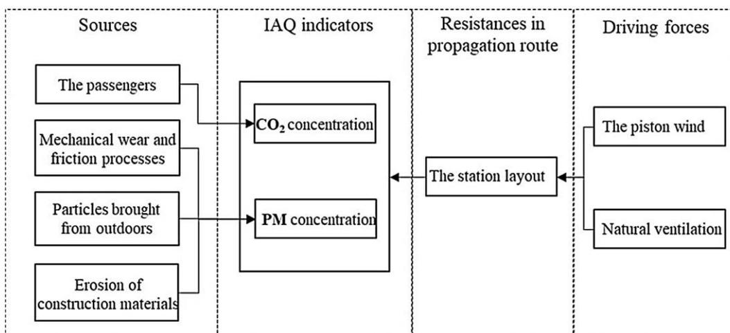
Figure 2: Schematic of IAQ influential factors for the public area.
