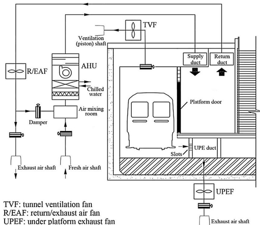
Figure 3: Schematic of a typical HVAC system in UMSs.
