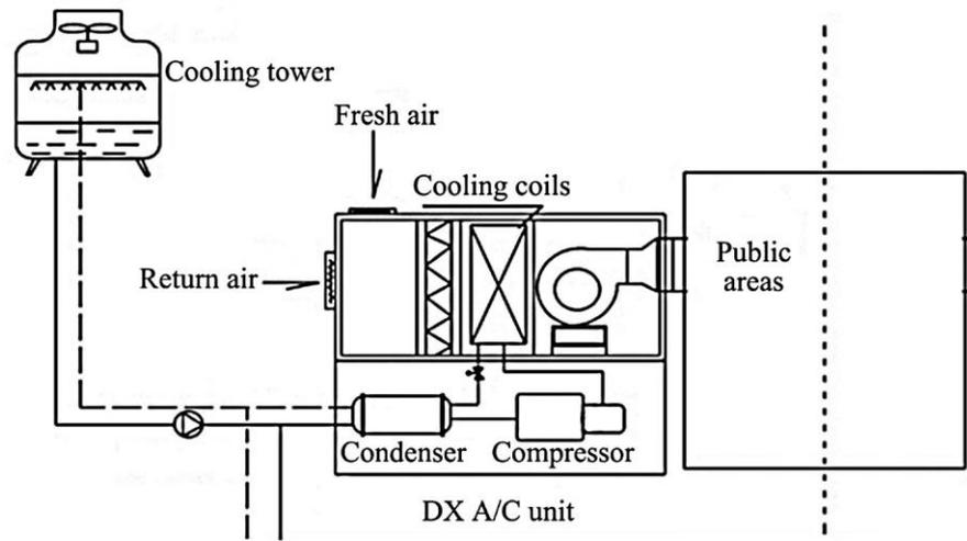
Figure 10: A schematic diagram for DX A/C systems.
