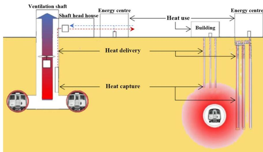
Figure 12: Heat recovery from tunnel air (left) and ground (right) (adapted from [87]).
