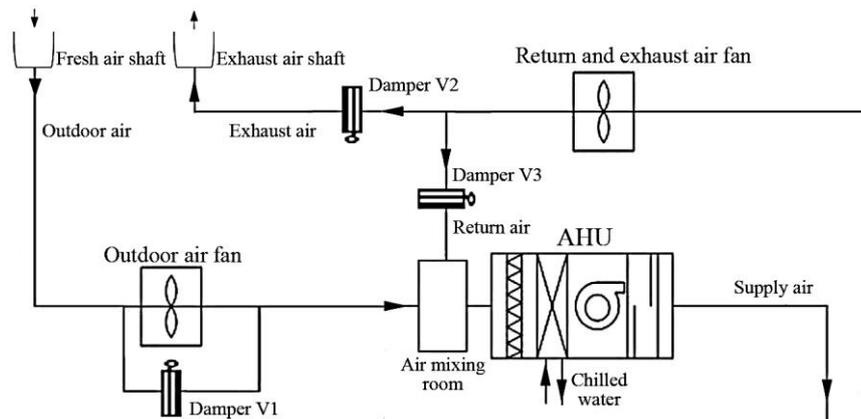
Figure 8: Air flow pattern in ventilation systems.
