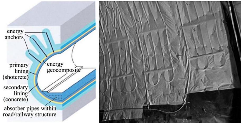
Figure 13: Schematic of an energy tunnel (adapted from [97]).
