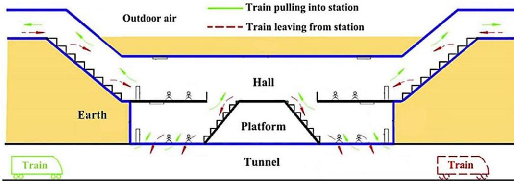
Figure 5: Air flow schematic of the piston effect in an island-type station (adapted from [53]).
