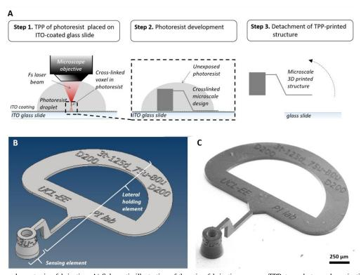
Fig. 3. Extrinsic sensor element microfabrication. A) Schematic illustration of the microfabrication process. TPP: two-photon polymerization, ITO-Indium Tin Oxide. B) Isometric view of the microstructure CAD of the consolidated design for TPP. C) SEM view of the TPP-fabricated microstructure following detachment from the glass substrate.
