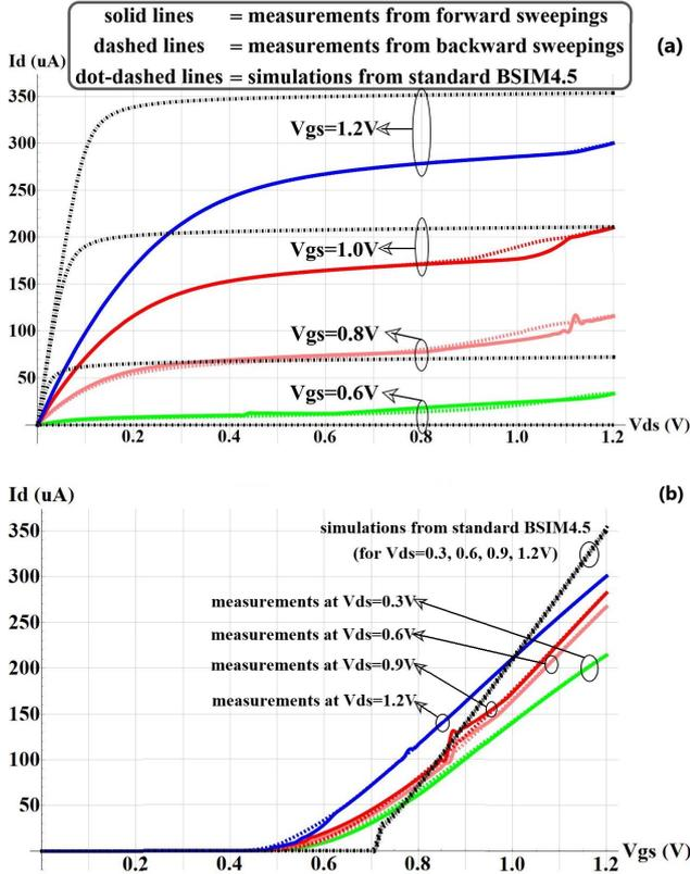
Fig. 1. Breakdown of simulations from BSIM4.5 model at LHT for characteristics of (a)  $I_d$ - $V_{ds}$  and (b)  $I_d$ - $V_{gs}$  for NMOS1.
