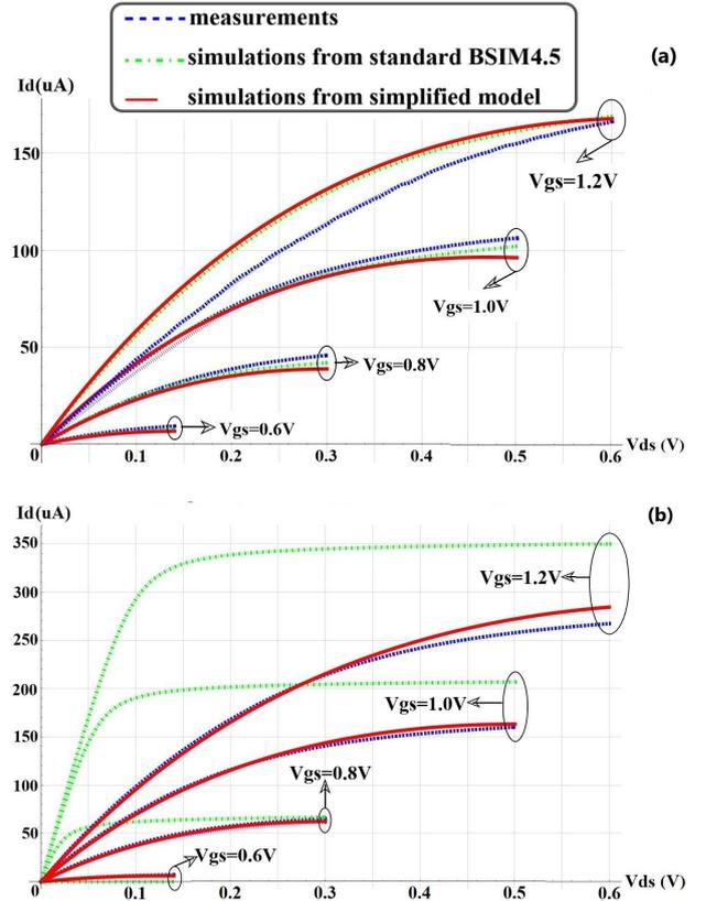
Fig. 2. Comparison between measurement and models at (a) RT and (b) LHT for NMOS1.
