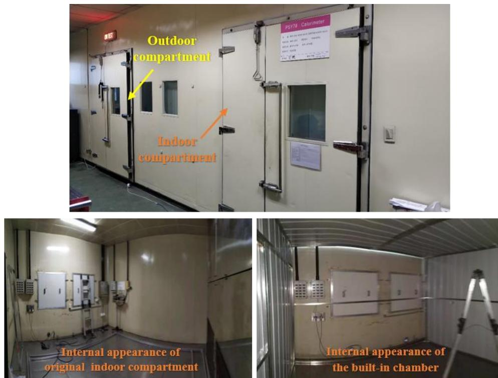
Fig. 1. The prototype of the calorimetric chamber.
