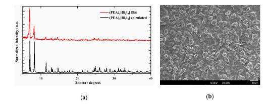
**Figure 1.** (a) Grazing Incidence X-ray diffraction (GIXRD) pattern of deposited (PEA)<sub>3</sub>Bi<sub>2</sub>I<sub>9</sub> film and standard powder XRD pattern calculated from single crystal XRD. (b) Top surface SEM image of (PEA)<sub>3</sub>Bi<sub>2</sub>I<sub>9</sub> film. Augmentation for the front view image is  $\times$ 2000.
