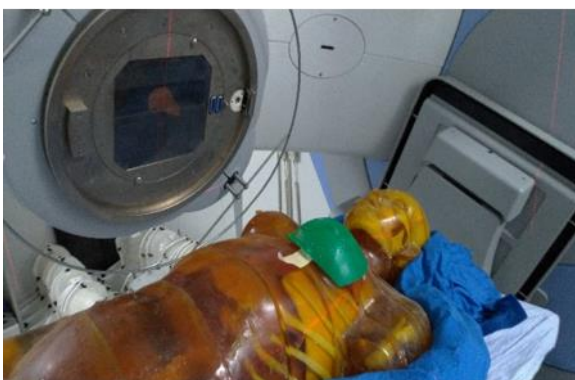
Figure 3.11: The setup of a female-phantom study and the location of TLD on the left breast of the phantom. S, I, R, L, and C refer to the superior side, inferior side, right side, left side, and centre point.
