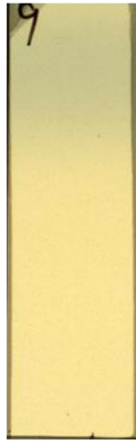
Figure 3.15: Demonstration of the irradiated strip with a 9 MeV electron beam. The beam enters from the side with a number, which is located in the darker part of the strip.
