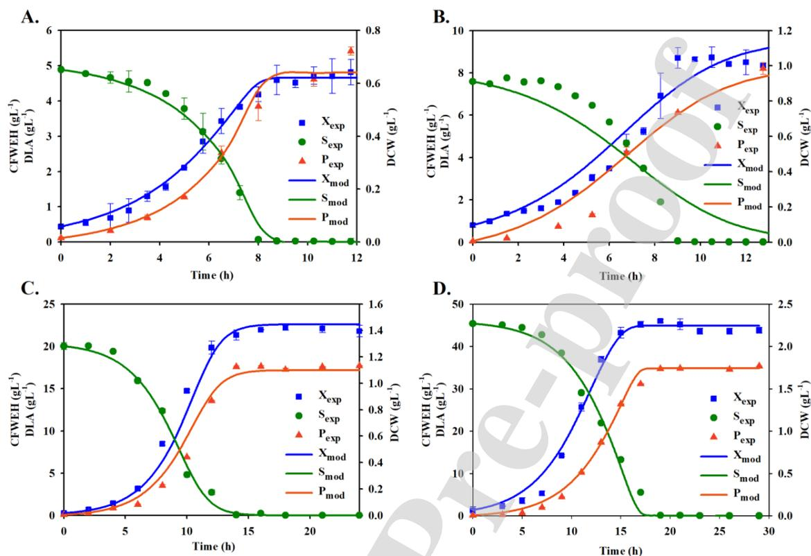
Figure 3. Comparison of experimental profiles of biomass (filled blue squares), CFWEH (filled green circles) and DLA (filled orange triangles) to the respective model predicted values of biomass (blue continuous), CFWEH (green continuous) and DLA (orange continuous) carried out by least square minimization method for different initial CFWEH concentrations: A. 5 gL<sup>-1</sup>; B. 8 gL<sup>-1</sup>; C. 20 gL<sup>-1</sup> D. 45 gL<sup>-1</sup>.
