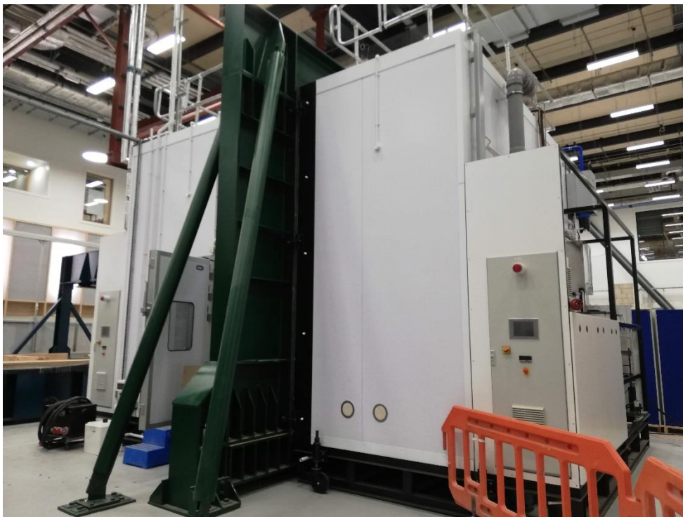
Figure 2: UCL CEGE External-Internal coupled environmental Chambers at UCL-Here East
