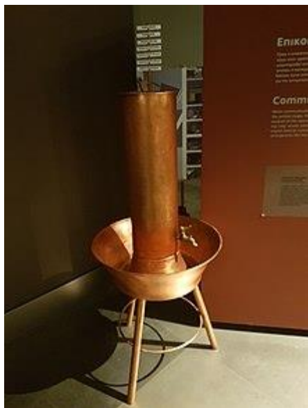
Figure 47a: Hydraulic Telegraph, reconstruction of the Thessaloniki Technology Museum
