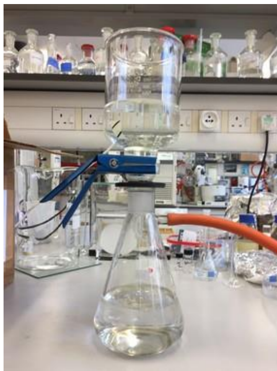
Figure 6.4. Picture of the HPLC filtration system used to filter water sample
