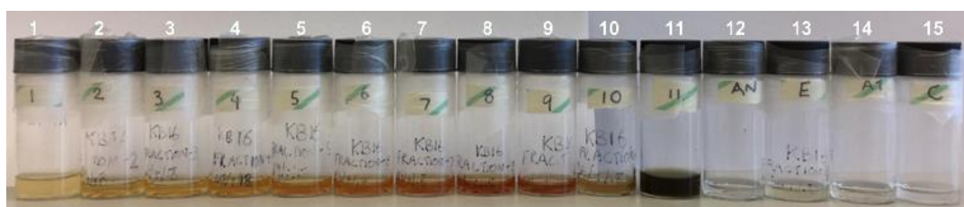
Figure 5.12. Each fraction after resuspension in solvent. Relative polarity of each fraction elute ranges from most polar (fraction 1) to least polar (fraction 15). The differences in colour across the fractions suggests that there may be a change in the content of the fractions.
