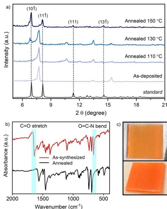
**Figure 4.** (a) GIXRD patterns of  $[\text{PEA}]_3[\text{Bi}_2]_9$  films deposited on glass and annealed in  $\text{N}_2$  at different temperatures in comparison to  $[\text{PEA}]_3[\text{Bi}_2]_9$  SCXRD standard; (b) FT-IR spectra of as-deposited and annealed in  $\text{N}_2$  (150 °C)  $[\text{PEA}]_3[\text{Bi}_2]_9$  thin films and (c) images of as-deposited (top) and annealed in  $\text{N}_2$  (150 °C) (bottom)  $[\text{PEA}]_3[\text{Bi}_2]_9$  coatings on glass.
