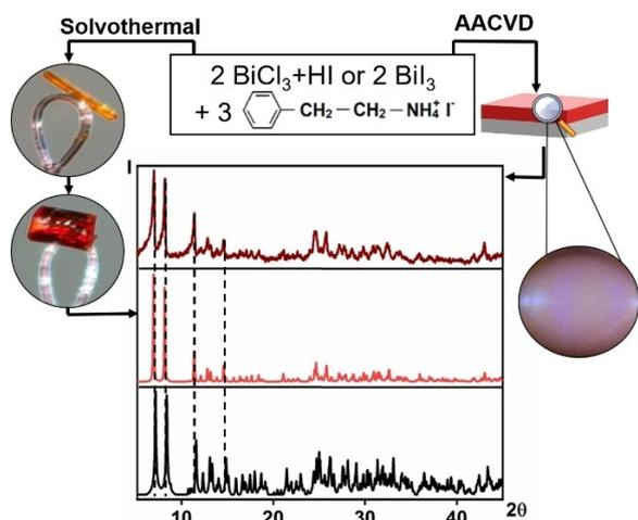
**Figure 2.** Synthesis methodologies employed to obtain  $[\text{PEA}]_3[\text{Bi}_2]_9$  single crystals and film coatings. PXRD patterns of scraped annealed film on glass (top) and calculated from SCXRD data (middle) are consistent with literature data (bottom).<sup>[23]</sup>
