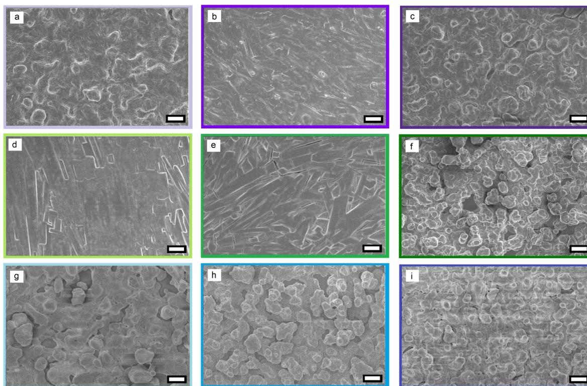
**Figure 5.** SEM images of hybrid thin films as-deposited (left column), vacuum annealed at 120 °C (middle column) and annealed in N<sub>2</sub> at 150 °C (right column) on FTO/glass substrates (purple, a–c), TiO<sub>2</sub>/glass (green, d–f) and float glass (blue, g–i). Magnification for all images is  $\times 1000$  and scale bar represents 10 μm.
