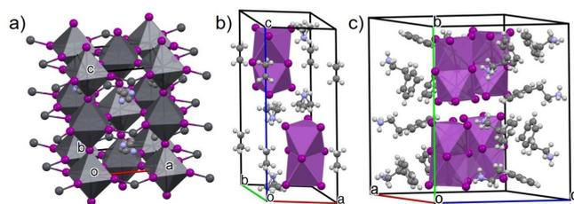
**Figure 1.** Unit cell of (a)  $\text{CH}_3\text{NH}_3\text{PbI}_3$ <sup>[35]</sup> (b)  $[\text{CH}_3\text{NH}_3]_3[\text{Bi}_2\text{I}_9]$ <sup>[33]</sup> and (c)  $[\text{C}_6\text{H}_5(\text{CH}_2)_2\text{NH}_3]_3[\text{Bi}_2\text{I}_9]$  (or  $[\text{PEA}]_3[\text{Bi}_2\text{I}_9]$ ) reproduced using Mercury®.
