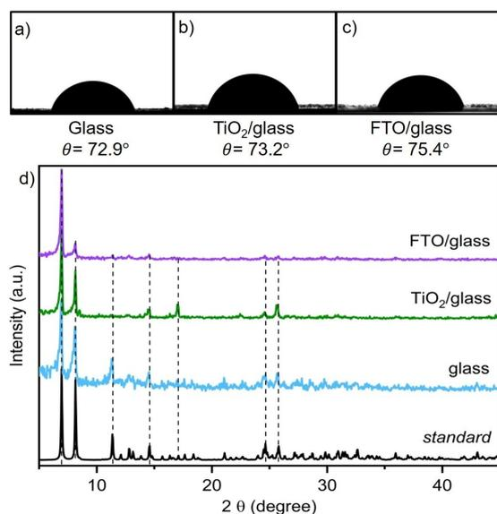
**Figure 7.** Water contact angles on vacuum annealed (120 °C)  $[\text{PEA}]_3[\text{Bi}_2\text{I}_9]$  thin films deposited over (a) float glass, (b)  $\text{TiO}_2/\text{glass}$  and (c)  $\text{FTO}/\text{glass}$ . (d) GIXRD patterns of vacuum annealed (120 °C)  $[\text{PEA}]_3[\text{Bi}_2\text{I}_9]$  thin films deposited over float glass (blue),  $\text{TiO}_2/\text{glass}$  (green) and  $\text{FTO}/\text{glass}$  (purple) after 6 months exposed to ambient conditions.
