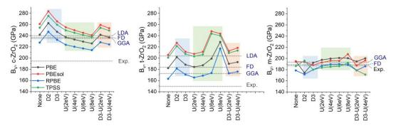
Figure 6. Computed bulk modulus B<sub>V</sub> (GPa) for (a) c<sub>7</sub>, (b) t<sub>7</sub>, and (c) m-ZrO<sub>2</sub>. Previously reported experimental<sup>57-59</sup> and theoretical (LDA,<sup>52</sup> GGA,<sup>14</sup> FD,<sup>7</sup> and LD<sup>60</sup>) values are also given for comparison. See Table S2-S4 (Supplementary Information).
