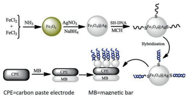
**Figure 17.** Schematic illustration of the fabrication of a DNA-biosensor based on MBCPE/ $\text{Fe}_3\text{O}_4@Ag$  composites. Reproduced with permission.<sup>[421]</sup> Copyright 2016, Elsevier.
