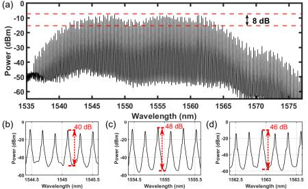
Fig. 3. (a) Measured spectrum of 26 GHz parametric frequency comb spanning more than 20nm, measured with 0.02 nm resolution. Close-in spectra measured at a resolution of 0.01nm are shown in insets below (b-d).
