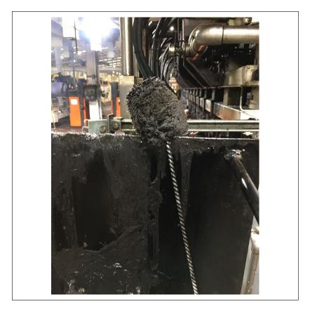
**Figure I.** A swabbing brush/stick used to apply oil (dobe) to the molds in the machinery that can be seen in the background of this photo.
