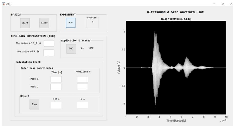
**Figure 1.** The user interface developed in MATLAB R2018a using the in-built GUIDE function. There is a control panel on the left-hand side and a display of the waveform on the right-hand side (voltage/amplitude against time).
