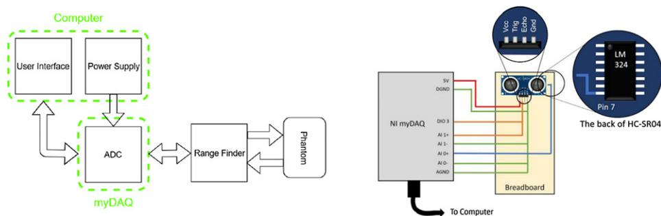
**Figure 2.** (a) (left) The block diagram of the toolkit. (b) (right) The schematic diagram showing the all of the wire connections between the range finder (HC-SR04) and NI myDAQ.
