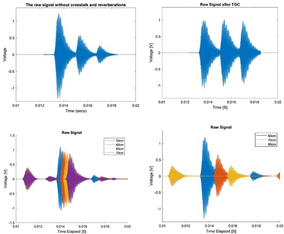
**Figure 4.** (a) (top left) The waveform plot before applying TGC algorithm. (b) (top right) The waveform plot after applying TGC algorithm. (c) (bottom left) The waveform plot showing resolvable peaks. Here the distance  $D$  between adjacent positions of the phantom is 20 cm and this is larger than the axial resolution of the range finder. (d) (bottom right) The waveform plot showing unresolvable peaks, with  $D = 5$  cm ( $D <$  axial resolution).
