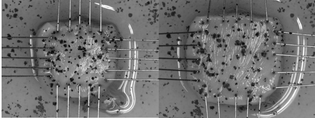
Figure 3.1: Mechanical testing of oesophageal sample loaded on CellScale biaxial testing system at 0% displacement (Left) and maximum displacement (Right).
