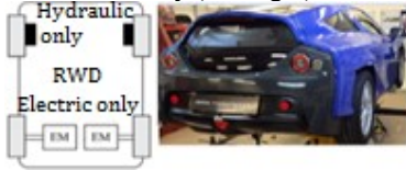
Fig.1. Experimental vehicle with novel brake-circuit configuration
