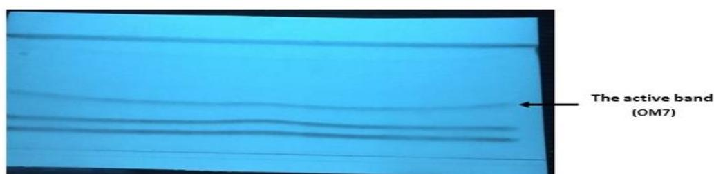
**Figure 2.11: RP-TLC (prep) of a compound OM7 under UV<sub>254</sub>.**
