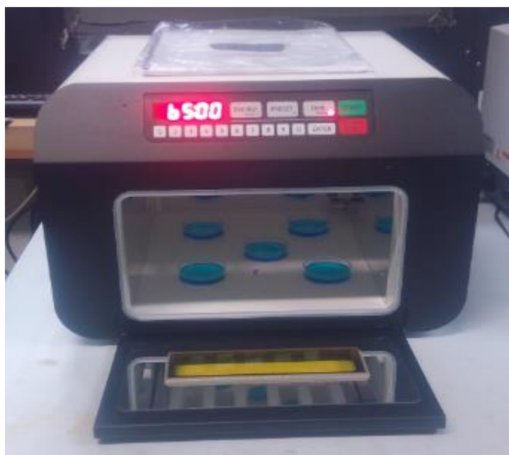
Figure 6-2 UV lamp used for preparation and photocatalytic test of polymer/TiO 2 composites.
