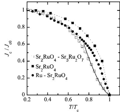
FIG. 2. Critical current density versus temperature for  $\text{Sr}_2\text{RuO}_4$ - $\text{Sr}_3\text{Ru}_2\text{O}_7$ ,  $\text{Sr}_2\text{RuO}_4$ , and  $\text{Ru-Sr}_2\text{RuO}_4$ . Critical current density is normalized to its value at 0.3 K. Temperature is normalized to  $T_c$ . The solid line shows a fit to the Ginzburg-Landau temperature dependence of  $J_c$  close to  $T_c$  in  $\text{Sr}_2\text{RuO}_4$ - $\text{Sr}_3\text{Ru}_2\text{O}_7$ .
