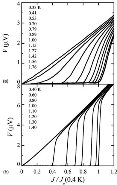
FIG. 1. Voltage versus critical current density for (a) the  $\text{Sr}_2\text{RuO}_4$ - $\text{Sr}_3\text{Ru}_2\text{O}_7$  eutectic and (b) pure  $\text{Sr}_2\text{RuO}_4$  with a  $T_c=1.35$  K. Current is applied along the  $c$  axis.
