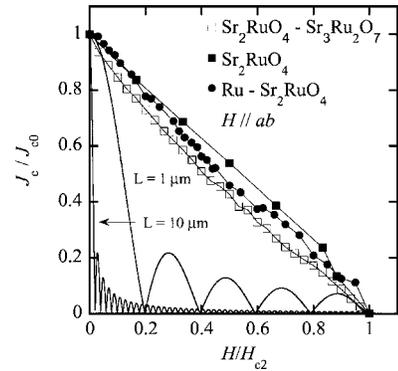
FIG. 3. Critical current density versus field for  $\text{Sr}_2\text{RuO}_4$ - $\text{Sr}_3\text{Ru}_2\text{O}_7$ ,  $\text{Sr}_2\text{RuO}_4$ , and  $\text{Ru-Sr}_2\text{RuO}_4$  for field in the  $ab$  plane. Critical current density is normalized to its value at 0 T, and the field is normalized to the upper critical field  $H_{c2}$ . The solid lines show the theoretical expectation for  $J_c(H)$  for an array of identical junctions, assuming junction lengths of 1 and 10  $\mu\text{m}$ .
