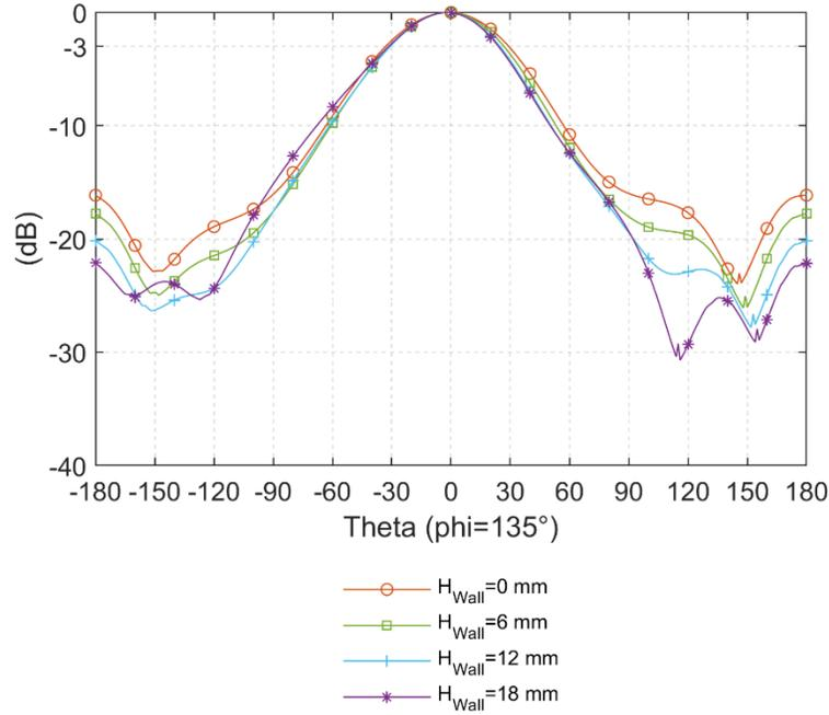
Fig. 4.50: Radiation pattern of the CP Pseudo-ME dipole antenna with different  $H_{Wall}$  when
