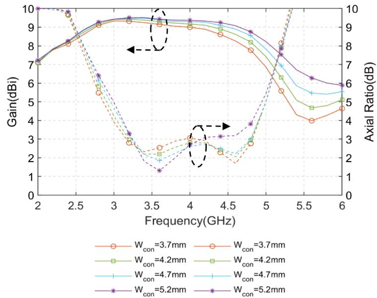
Fig. 4.17: Simulated gain and the axial ratio of the proposed CP Pseudo-ME dipole antenna with different  $W_{Con}$
