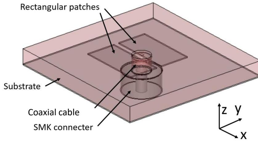
Fig. 5.1: Geometry of Model A
