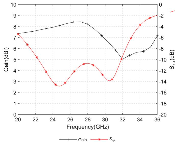
Fig. 5.2: Simulated gain and  $S_{11}$  of Model A
