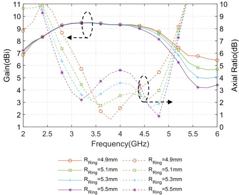
Fig. 4.23: Simulated gain and the axial ratio of the proposed CP Pseudo-ME dipole antenna with different  $R_{Ring}$
