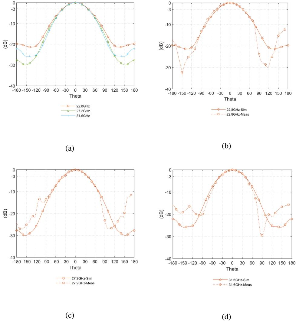
Fig. 5.34: H-plane radiation patterns of the proposed mmW antenna at different frequencies.
