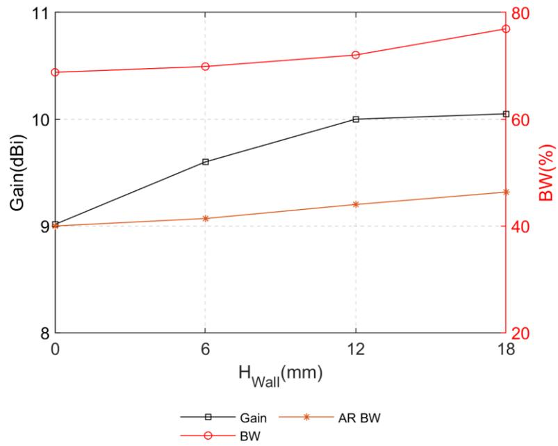
Fig. 4.51: Average gain, impedance bandwidth and axial ratio bandwidth with different  $H_{Wall}$
