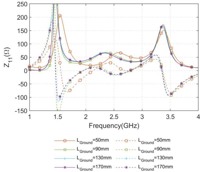
Fig. 3.10:  $Z_{11}$  of the cavity-less Pseudo-ME dipole antenna at the different ground size ( $L_{Ground}$ )
