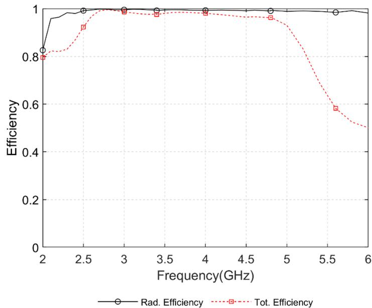
Fig. 4.36: Simulated radiation and total efficiency of the CP ME dipole
