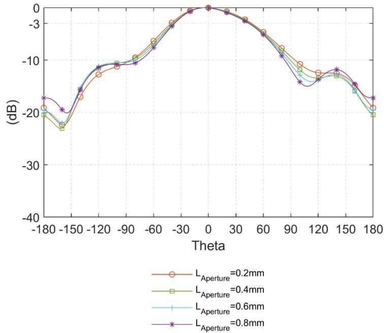
Fig. 5.19: E-plane radiation pattern at 27.5 GHz with different  $L_{Aperture}$
