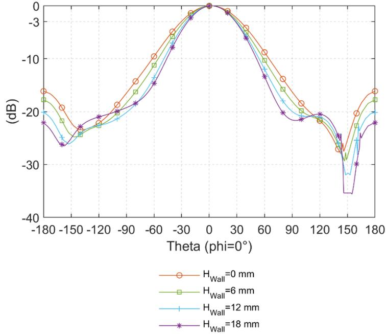
Fig. 4.47: Radiation pattern of the CP Pseudo-ME dipole antenna with different  $H_{Wall}$  when
