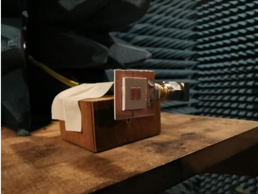
Fig. 5.30: Final prototype antenna under test in the anechoic chamber
