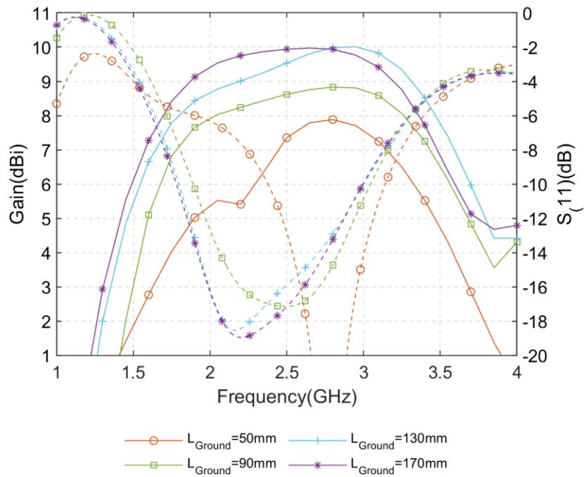
Fig. 3.11: Gain and  $S_{11}$  of the cavity-less Pseudo-ME dipole with different ground size ( $L_{Ground}$ )
