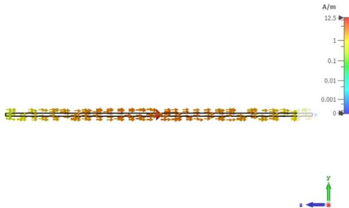
Fig. 2.8: The current distribution along a half-wave dipole at phase equals  $90^\circ$
