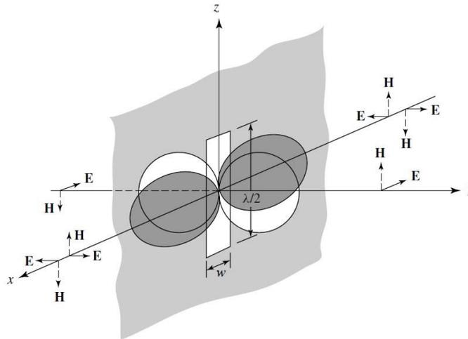
Fig. 2.15: Radiation fields of a magnetic dipole
