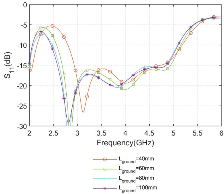
Fig. 4.27: Simulated  $S_{11}$  of the proposed CP Pseudo-ME dipole antenna with different  $L_{Ground}$
