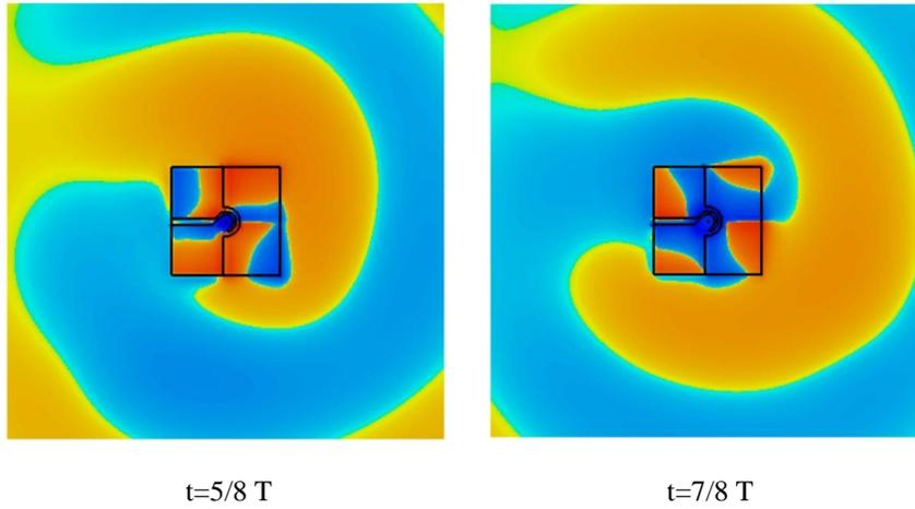
Fig. 4.10: E-field z-axis components distribution at different time
