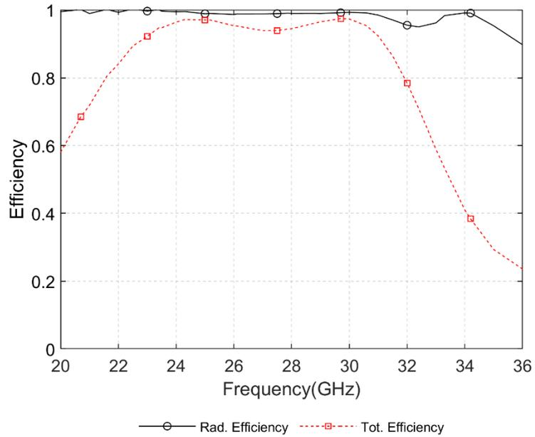
Fig. 5.32: Simulated radiation and total efficiency of the CP ME dipole
