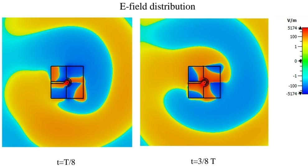
*Crossed-dipole Feed Circularly Polarized Pseudo Magneto-electric dipole Antenna-Operation Principle*
