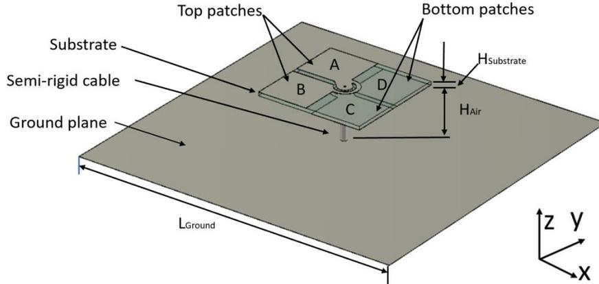
Fig. 4.1: The geometry of the crossed-dipole feed circularly polarized ME dipole
