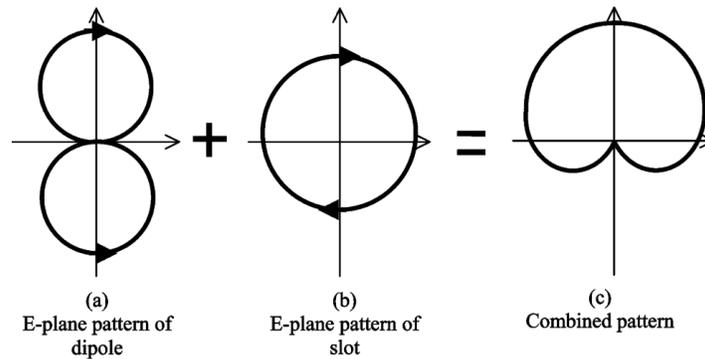
Fig. 2.16: E-plane radiation pattern of combined electric dipole and magnetic dipole [24]
