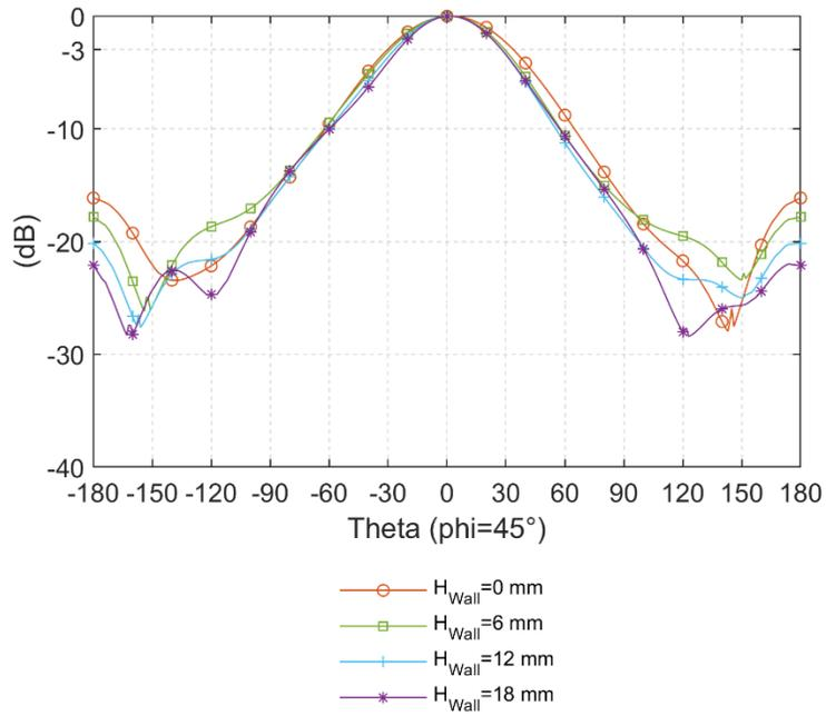
Fig. 4.48: Radiation pattern of the CP Pseudo-ME dipole antenna with different H<sub>Wall</sub> when
