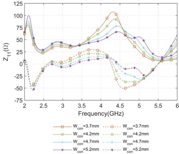
Fig. 4.16: Simulated  $Z_{11}$  of the proposed CP Pseudo-ME dipole antenna with different  $W_{Con}$
