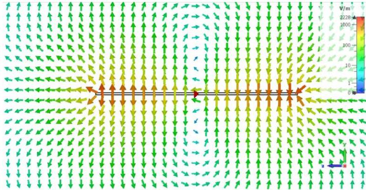
Fig. 2.9: The electric field of electric dipole when phase equal to  $0^\circ$
