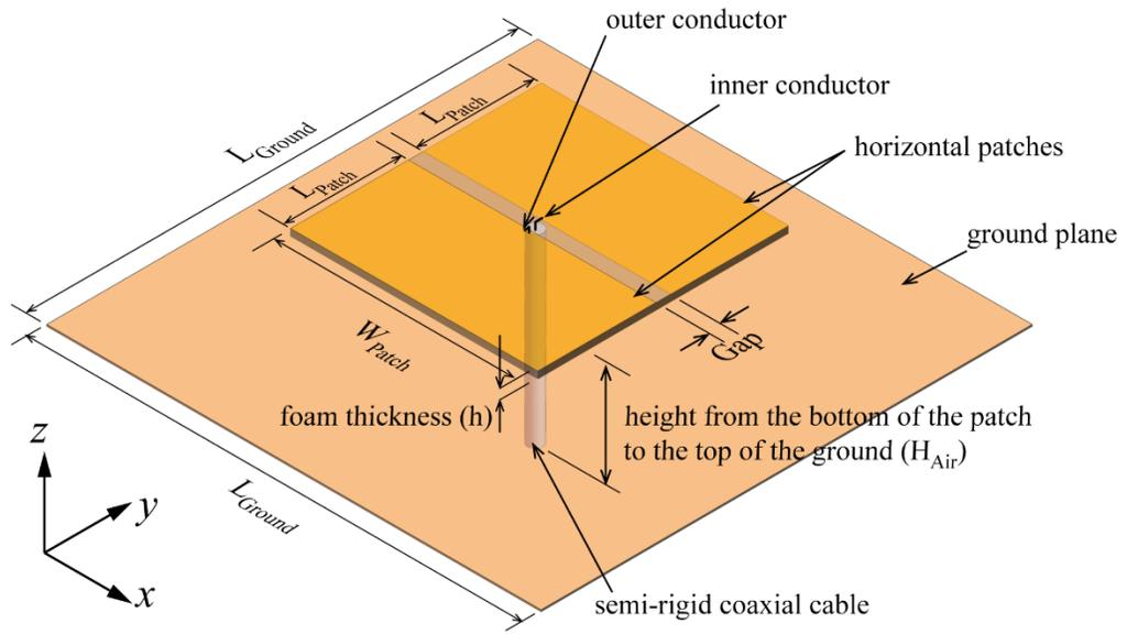
Fig. 3.1: The geometry of the cavity-less Pseudo-ME dipole antenna.
