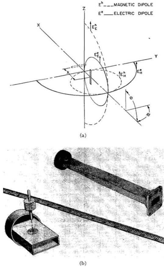
Fig. 2.17: (a). Electric and magnetic field distribution for two complementary dipoles (b). Test feed [12]
