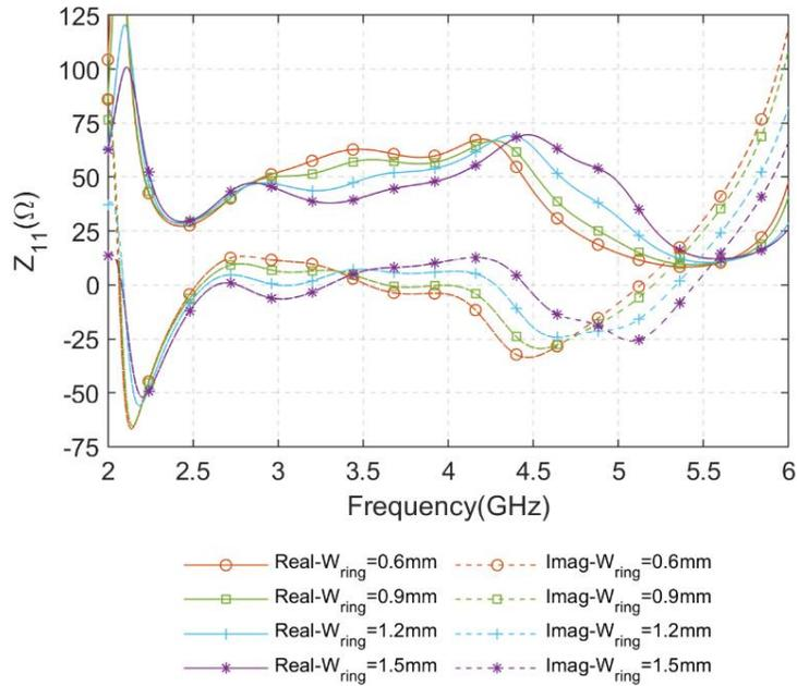
Fig. 4.19: Simulated  $Z_{11}$  of the proposed CP Pseudo-ME dipole antenna with different  $W_{Ring}$
