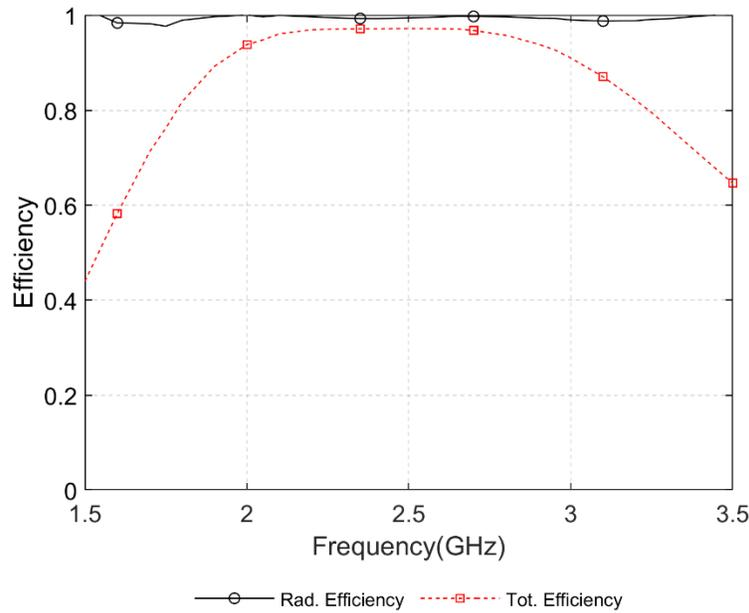
Fig. 3.17: Simulated radiation and total efficiency of the proposed cavity-less ME dipole
