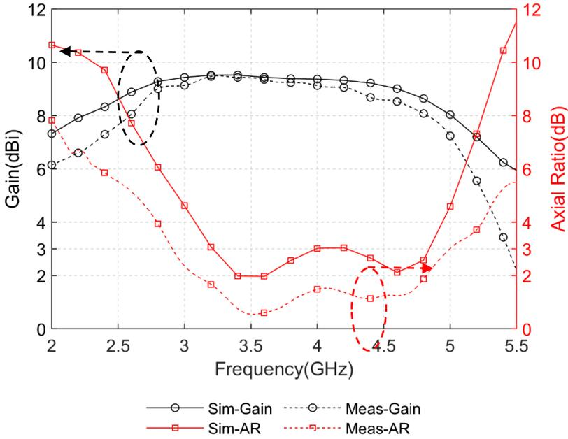
Fig. 4.35: Simulated and measured gain and the axial ratio of the CP ME dipole
