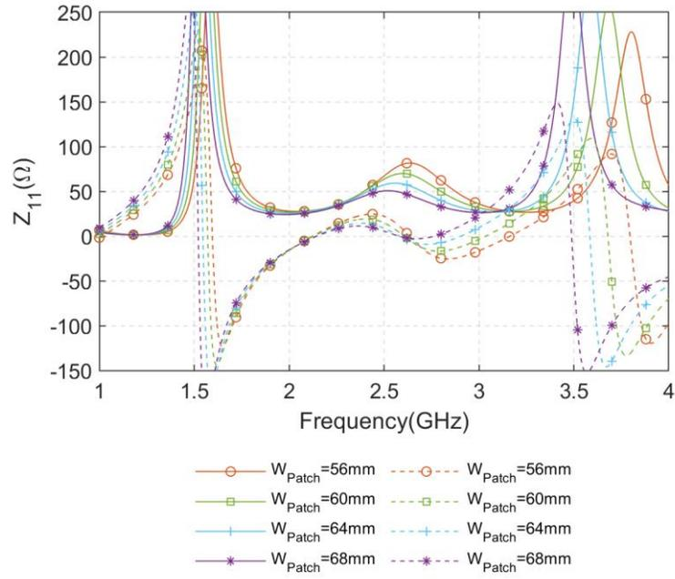
Fig. 3.6:  $Z_{11}$  of the cavity-less Pseudo-ME dipole antenna at different patch width ( $W_{Patch}$ )
