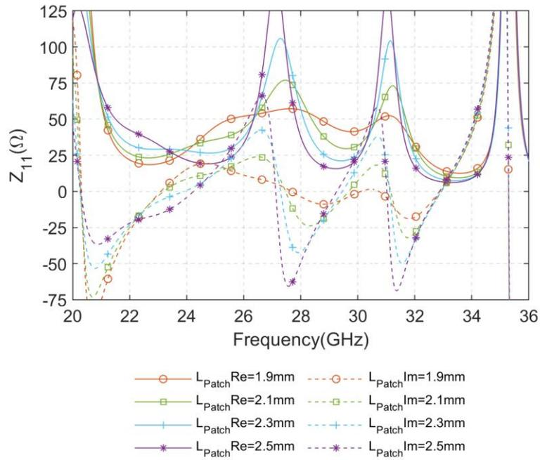
Fig. 5.14: Simulated  $Z_{11}$  of the proposed mmW Pseudo-ME dipole antenna with different  $L_{Patch}$
