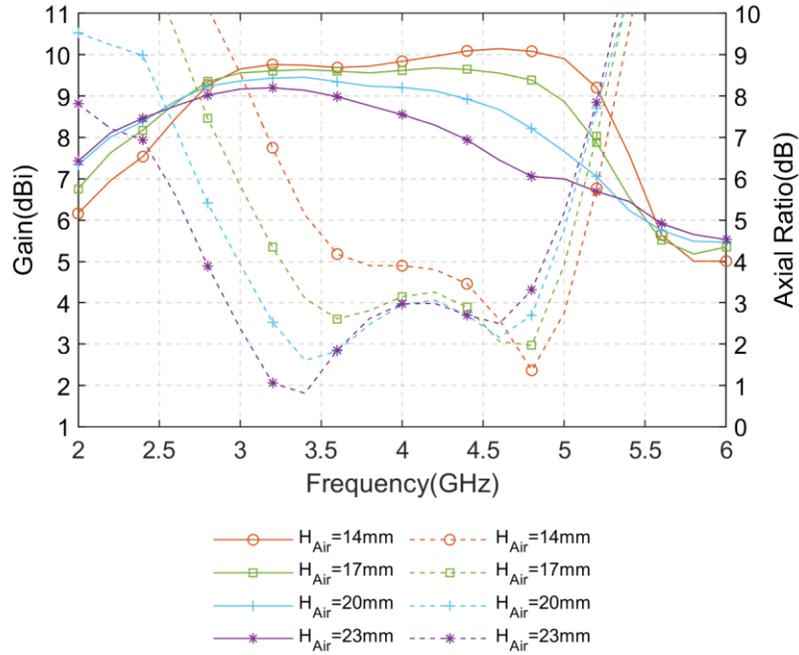
Fig. 4.26: Simulated gain and the axial ratio of the proposed CP Pseudo-ME dipole antenna with different  $H_{Air}$
