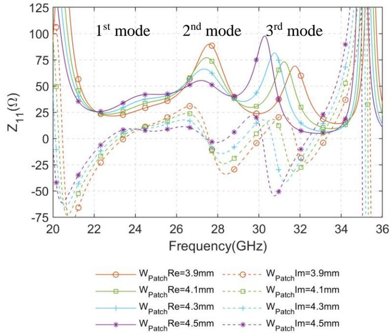
Fig. 5.12: Simulated  $Z_{11}$  of the mmW Pseudo-ME dipole antenna with different  $W_{Patch}$
