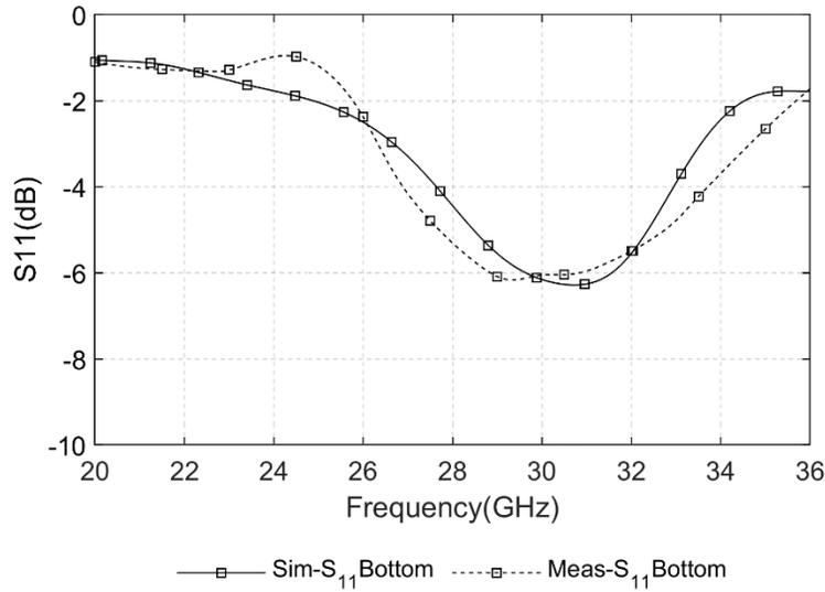
Fig. 5.8: Comparison of measured and simulated  $S_{11}$  of the bottom layer millimeter-wave Pseudo-ME dipole
