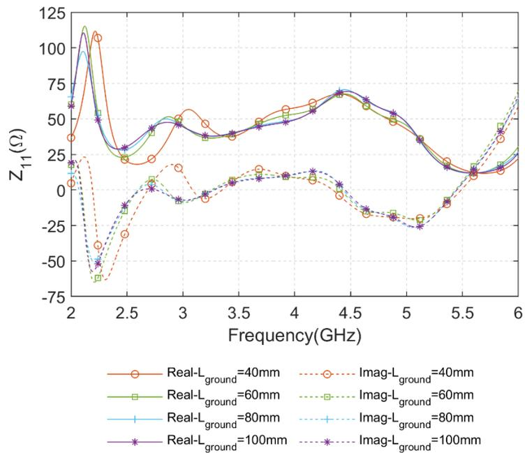
Fig. 4.28: Simulated  $Z_{11}$  of the proposed CP Pseudo-ME dipole antenna with different  $L_{Ground}$
