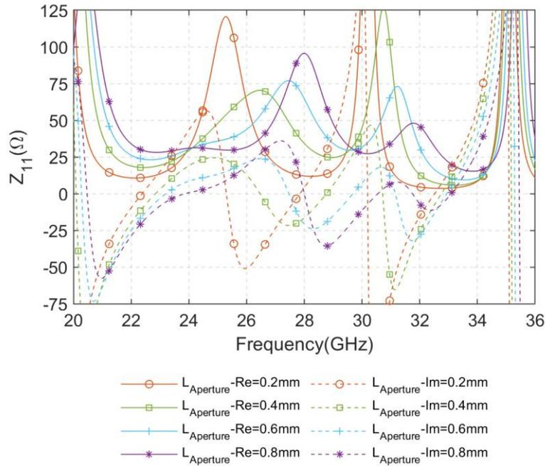
Fig. 5.18: Simulated  $Z_{11}$  of the proposed mmW Pseudo-ME dipole antenna with different
