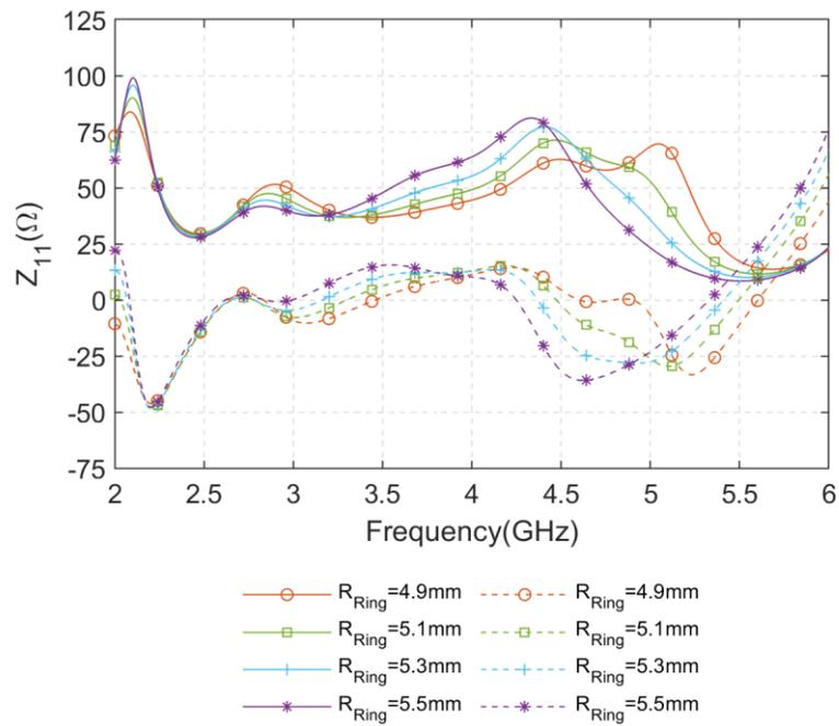
Fig. 4.22: Simulated  $Z_{11}$  of the proposed CP Pseudo-ME dipole antenna with different  $R_{Ring}$
