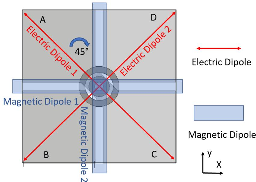
Fig. 4.3: The four fundamental mode of the crossed-dipole feed CP pseudo-ME dipole antenna
