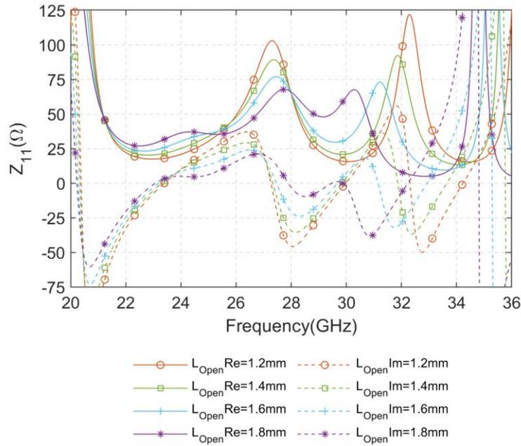
Fig. 5.28: Simulated  $Z_{11}$  of the mmW Pseudo-ME dipole antenna with different  $L_{Open}$
