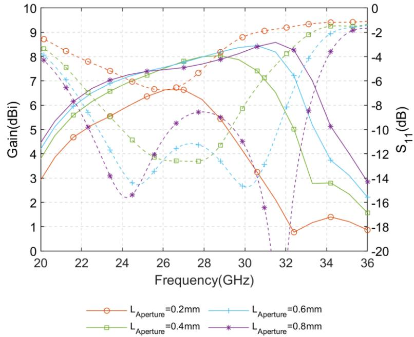
Fig. 5.17: Simulated  $S_{11}$  and gain of the mmW Pseudo-ME dipole antenna with different
