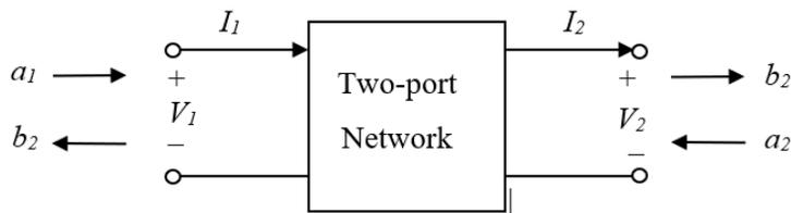
Fig. 2.2: Two-port network inputs and outputs
