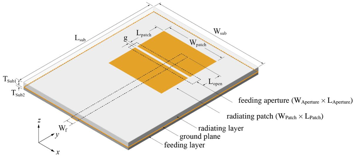
Fig. 5.4: The geometry of the aperture-coupled millimeter-wave Pseudo-ME dipole antenna.
