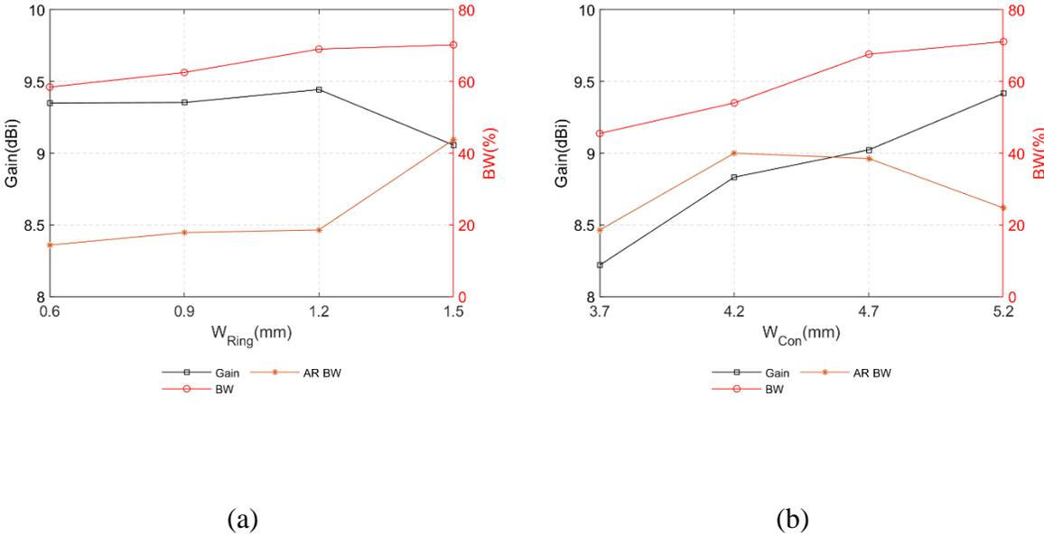
*Crossed-dipole Feed Circularly Polarized Pseudo Magneto-electric dipole Antenna-Parametric Study*
