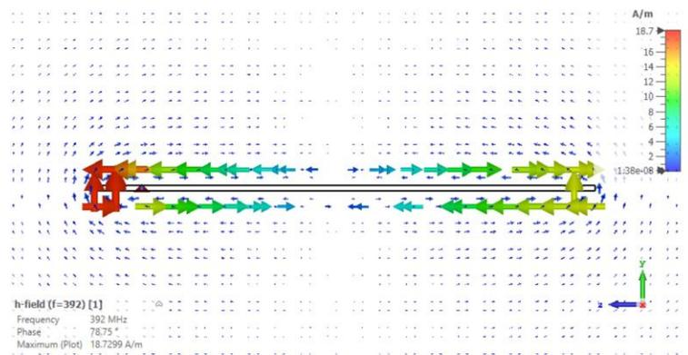
Fig. 2.14: The current distribution along with the slot
