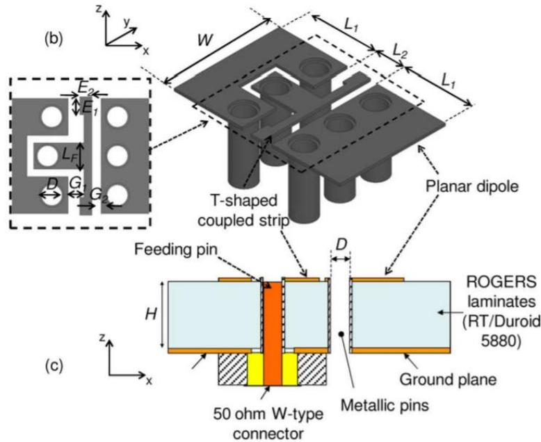
Fig. 2.20: 3-D view and side view of the 60-GHz printed ME dipole antenna [45]
