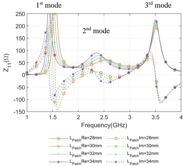
Fig. 3.4:  $Z_{11}$  of the cavity-less Pseudo-ME dipole antenna at different patch length ( $L_{Patch}$ )
