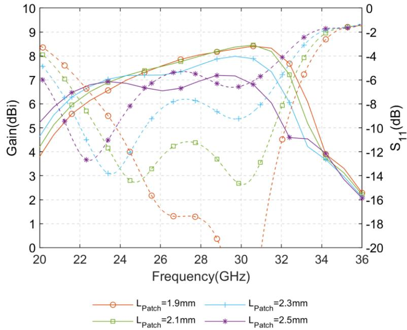
Fig. 5.13: Simulated  $S_{11}$  and gain of the mmW Pseudo-ME dipole antenna with different  $L_{Patch}$
