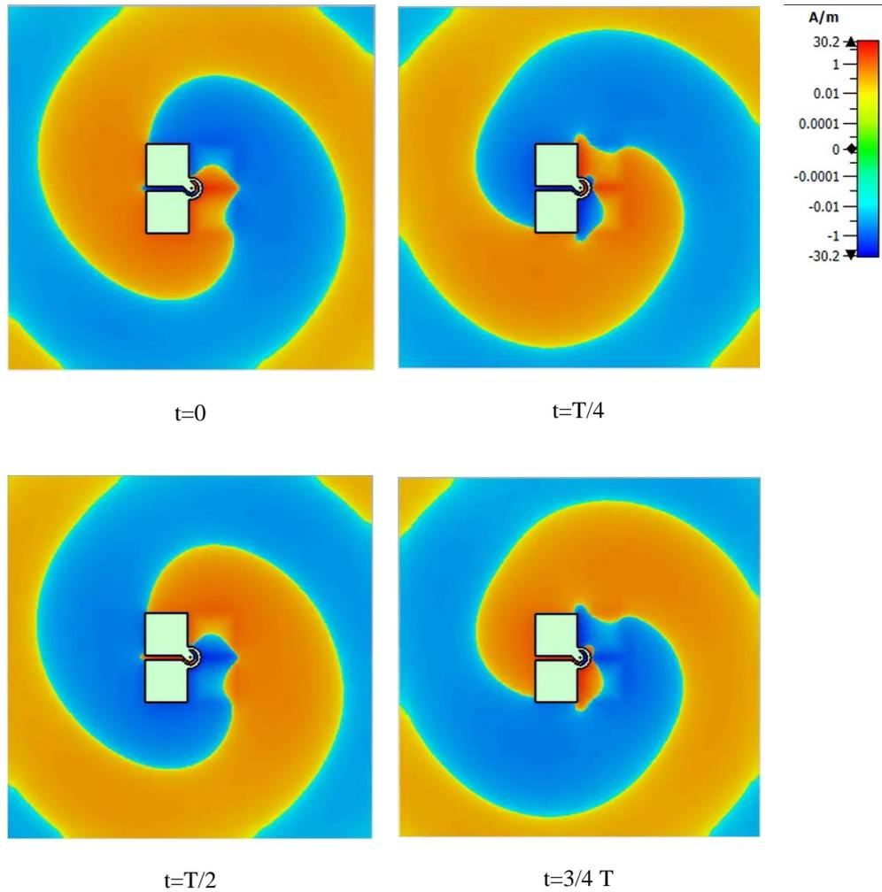
Fig. 4.8: H-field z-axis components distribution at different time
