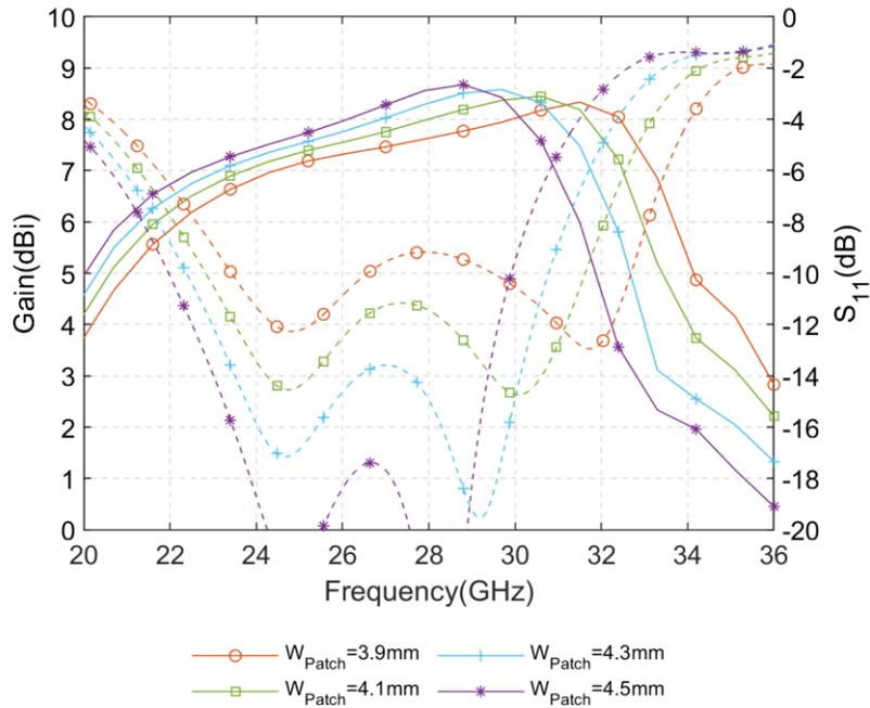
Fig. 5.11: Simulated  $S_{11}$  and gain of the mmW Pseudo-ME dipole antenna with different  $W_{Patch}$
