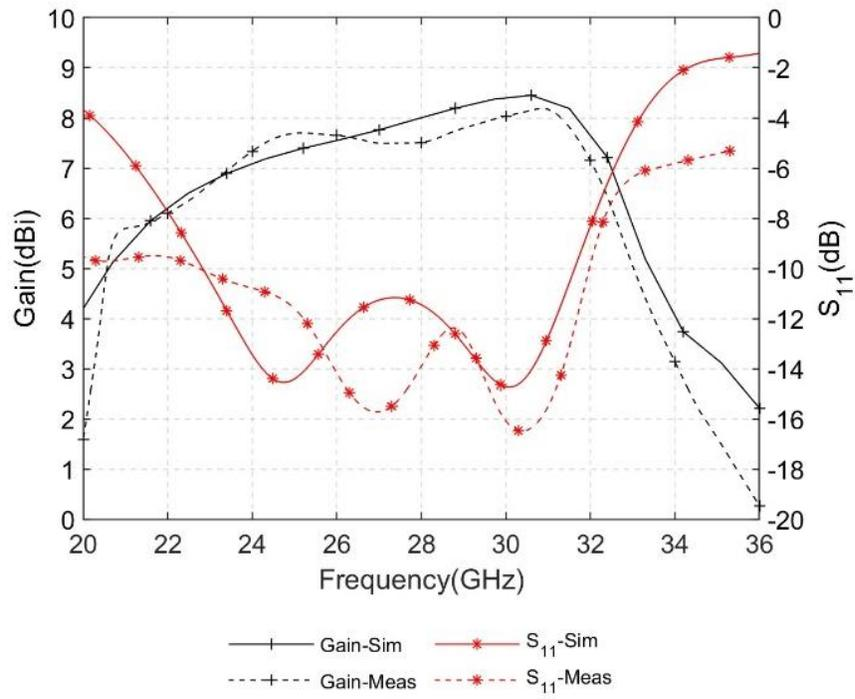
Fig. 5.31: Simulated Gain and  $S_{11}$  of the proposed antenna.
