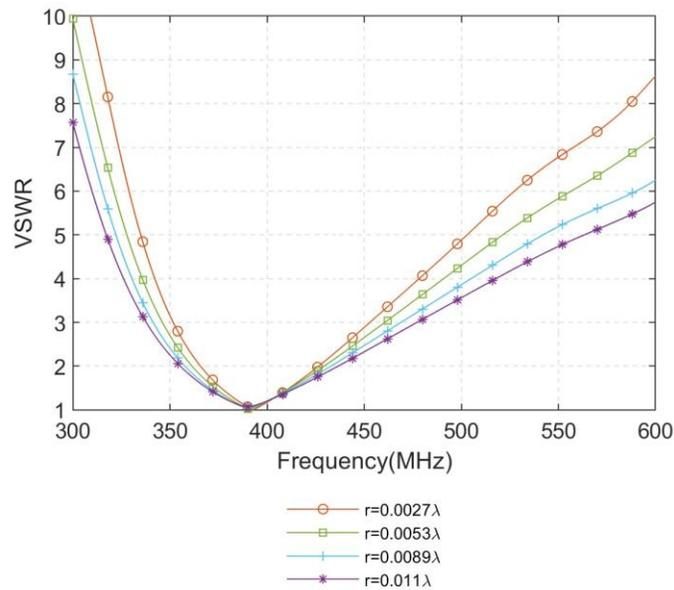
Fig. 2.11: VSWR of a half-wave dipole with different radius
