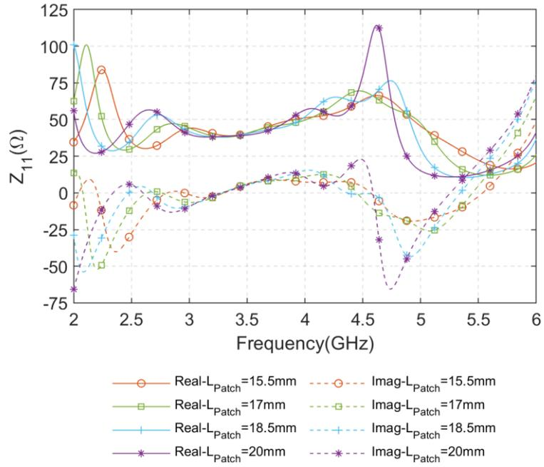
Fig. 4.12: Simulated  $Z_{11}$  and gain of the proposed CP pseudo-ME dipole antenna with different
