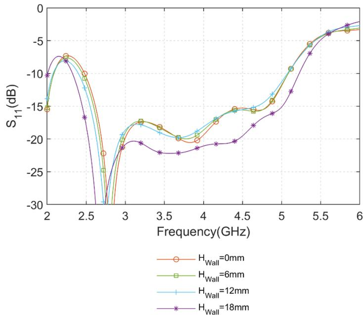
Fig. 4.44: Simulated  $S_{11}$  of the proposed antenna with different  $H_{Wall}$
