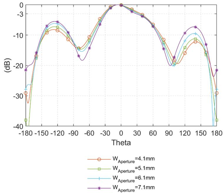
Fig. 5.25: E-plane radiation pattern of at 27.5 GHz with different  $W_{\text{Aperture}}$
