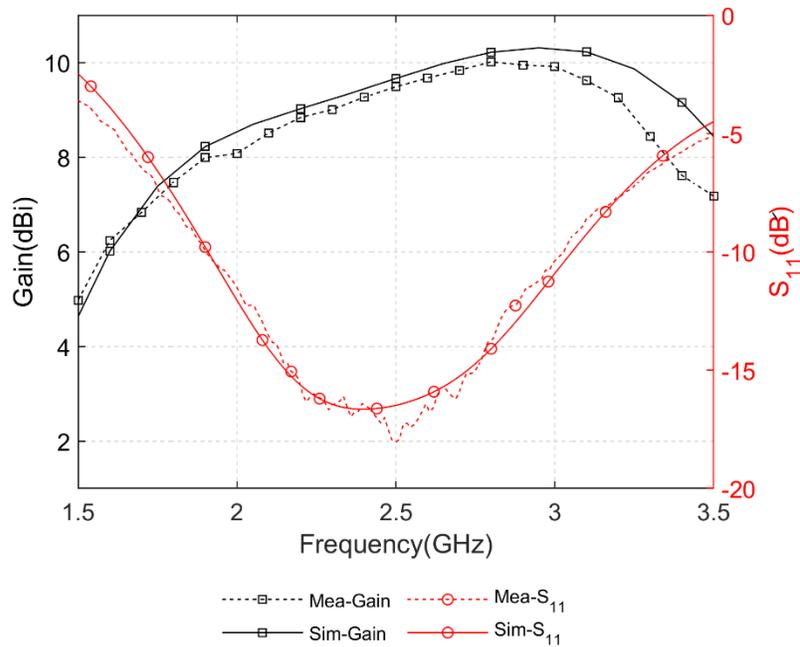
Fig. 3.16: Simulated and measured gain and  $S_{11}$  of cavity-less ME dipole
