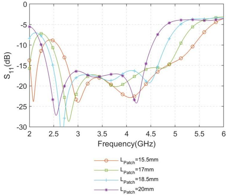
Fig. 4.13: Simulated  $S_{11}$  of the proposed CP Pseudo-ME dipole antenna with different  $L_{Patch}$
