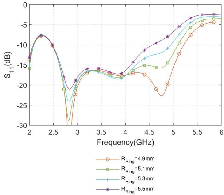
Fig. 4.21: Simulated  $S_{11}$  of the proposed CP Pseudo-ME dipole antenna with different  $R_{Ring}$
