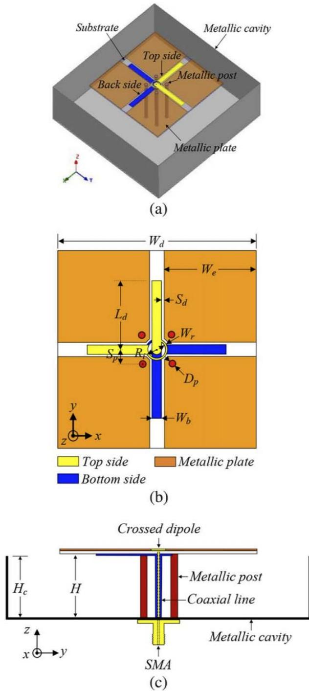
Fig. 2.21: The geometry of the crossed dipole loaded with Pseudo-ME dipole [35]
