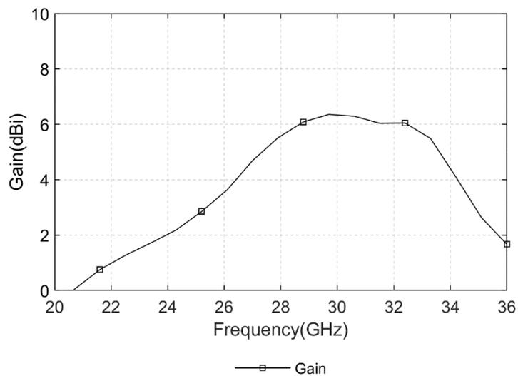
Fig. 5.10: Simulated gain of the transmitting layer
