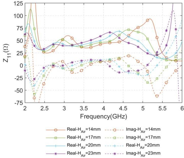
Fig. 4.25: Simulated  $Z_{11}$  of the proposed CP Pseudo-ME dipole antenna with different  $H_{Air}$
