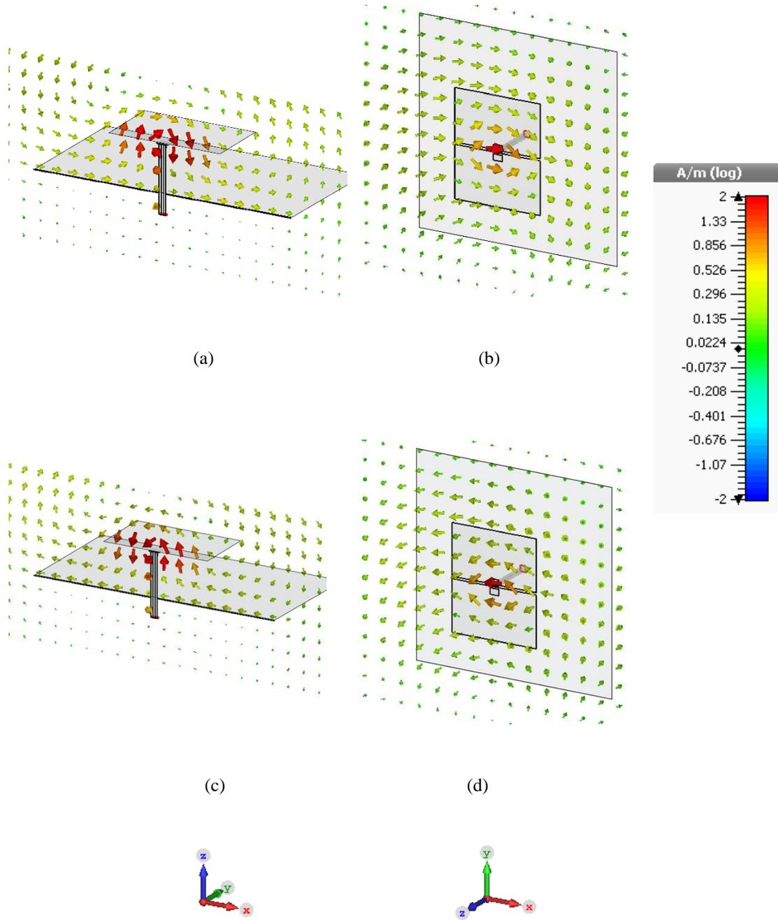
Fig. 3.3: H-field of magnetic dipole mode. xz plane cut. (a)  $t = T/4$ ; (b)  $t = T/4$ ; xy plane cut (c)  $t = 3T/4$ ; (d)  $t = 3T/4$
