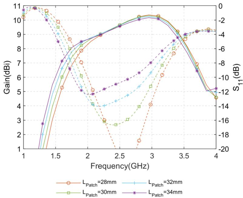
Fig. 3.5: Gain and  $S_{11}$  of the cavity-less Pseudo-ME dipole antenna at different patch length
