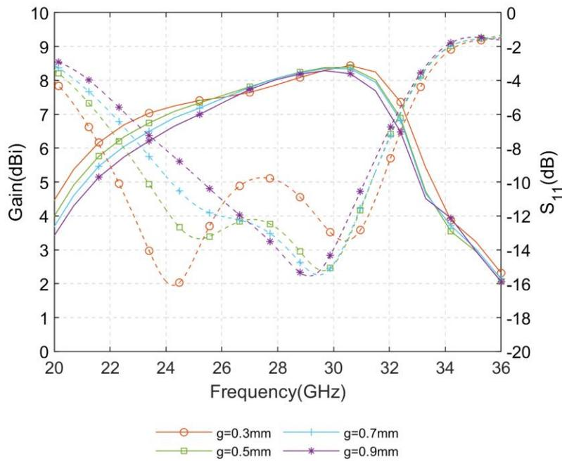
Fig. 5.15: Simulated  $S_{11}$  and gain of the proposed mmW Pseudo-ME dipole antenna with different  $g$
