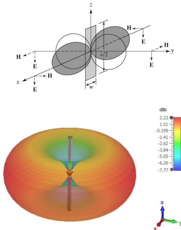
Fig. 2.10: The Radiation pattern of a half-wave dipole in three dimensions
