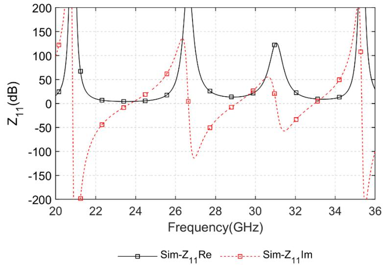
Fig. 5.9: Simulated  $Z_{11}$  of the bottom layer millimeter-wave Pseudo-ME dipole
