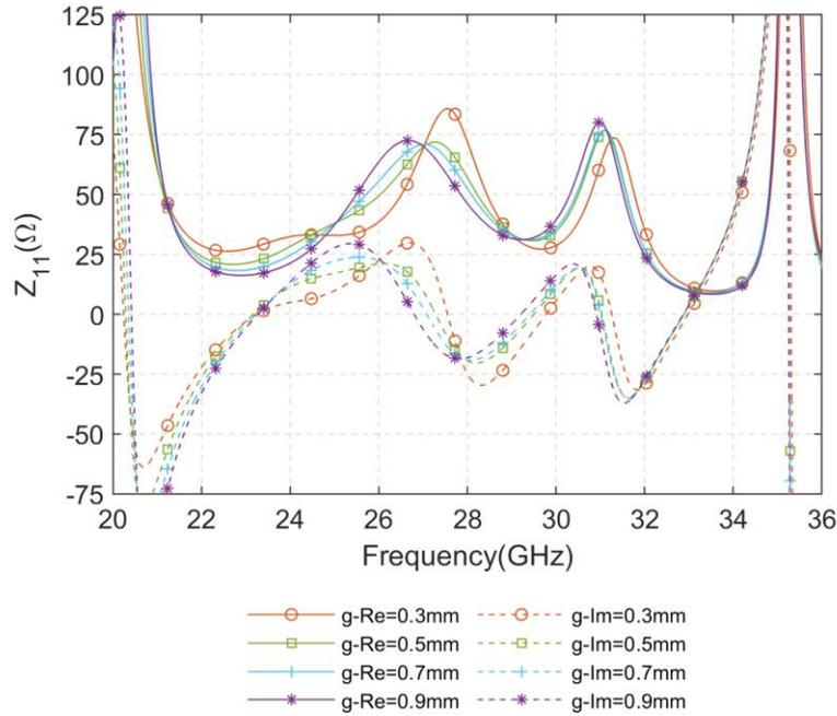
Fig. 5.16: Simulated  $Z_{11}$  of the proposed mmW Pseudo-ME dipole antenna with different  $g$
