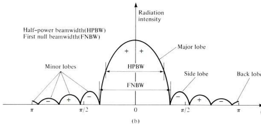
Fig. 2.4: Linear plot of radiation pattern [2]
