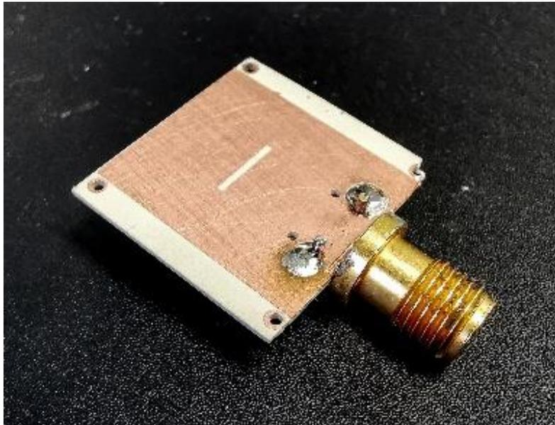
Fig. 5.7: The bottom layer of the millimeter-wave Pseudo-ME dipole (second attempt)
