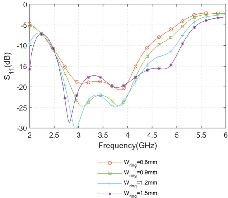
Fig. 4.18: Simulated  $S_{11}$  of the proposed CP Pseudo-ME dipole antenna with different  $W_{\text{Ring}}$
