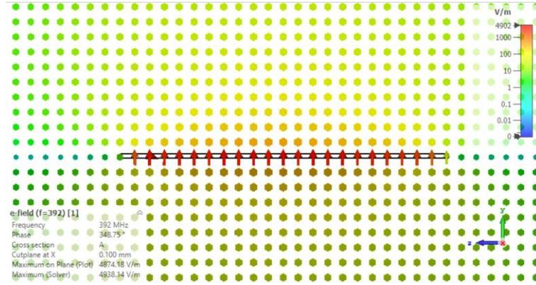
Fig. 2.13: The electric field along with the slot when phase equal to  $0^\circ$
