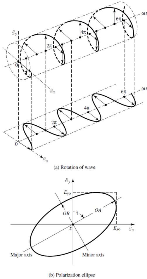
Fig. 2.5: (a) The electric field of circular polarization. (b). Elliptical polarization [16]
