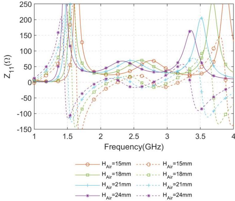
Fig. 3.8:  $Z_{11}$  of the cavity-less Pseudo-ME dipole antenna at a different height ( $H_{Air}$ )
