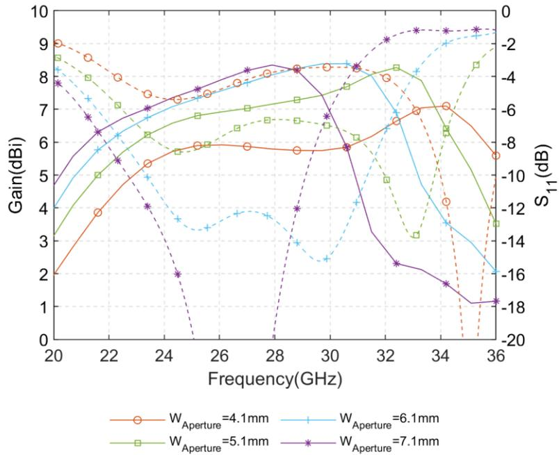
Fig. 5.22: Simulated  $S_{11}$  and gain of the mmW Pseudo-ME dipole antenna with different
