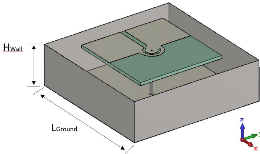
Fig. 4.43: The geometry of the CP Pseudo-ME dipole antenna with the metallic cavity
