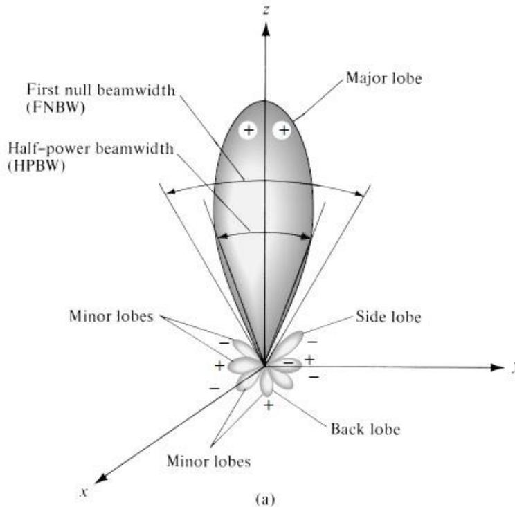
Fig. 2.3: Radiation pattern in three-dimension [16]
