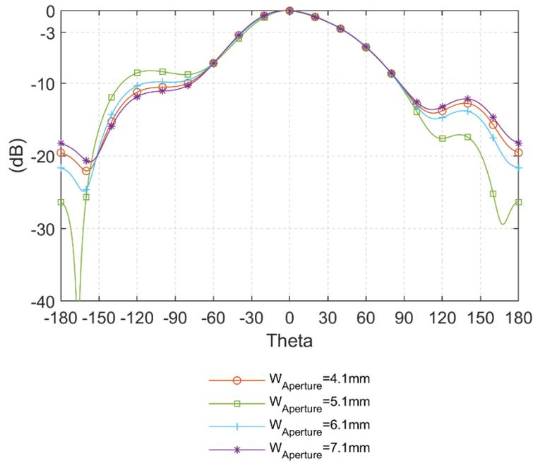
Fig. 5.24: E-plane radiation pattern of at 22.8 GHz with different  $W_{\text{Aperture}}$
