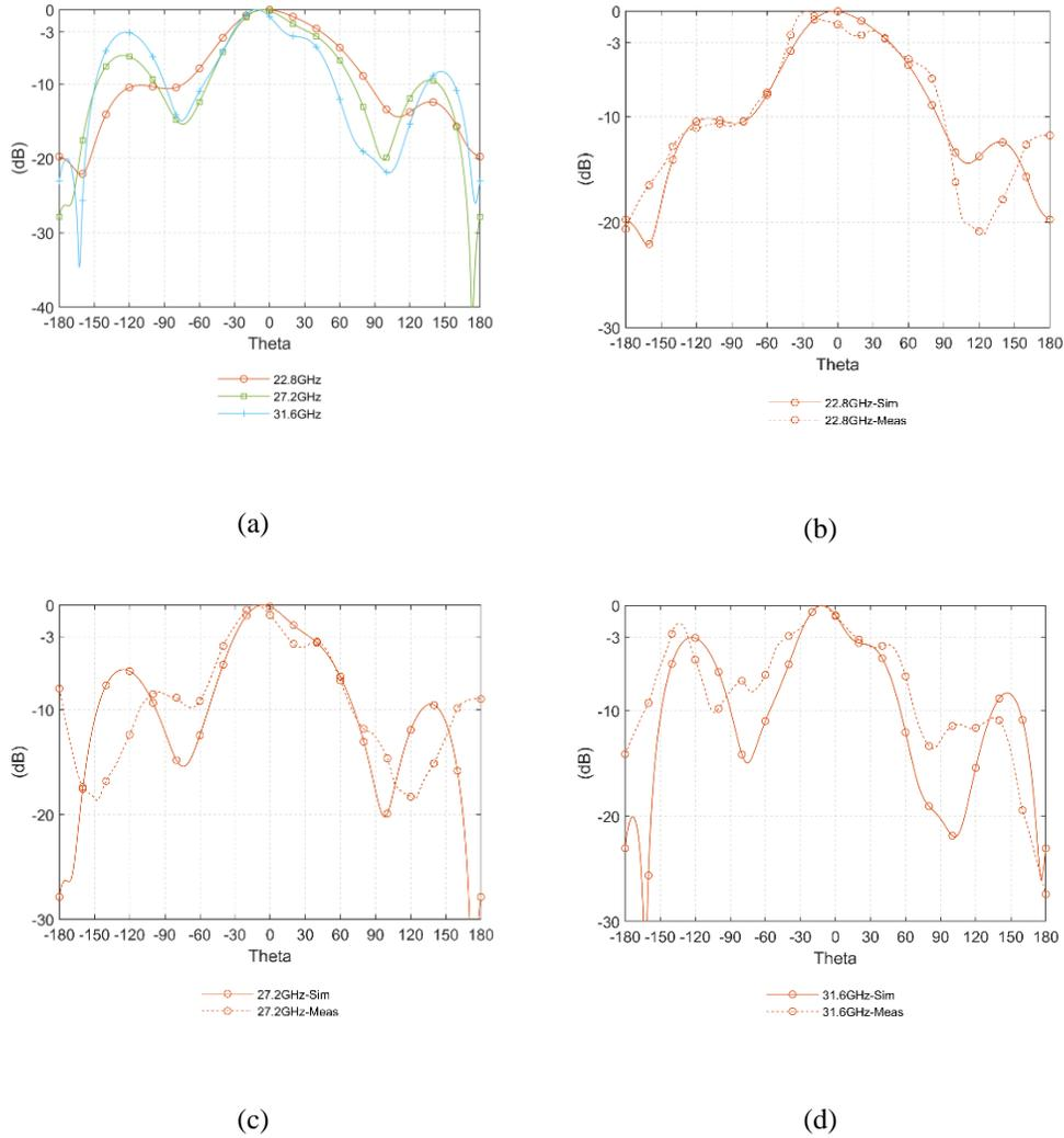
Fig. 5.33: E-plane radiation patterns of the proposed mmW antenna at different frequencies
