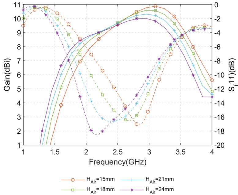
Fig. 3.9: Gain and  $S_{11}$  of the cavity-less Pseudo-ME dipole antenna at a different height ( $H_{Air}$ )
