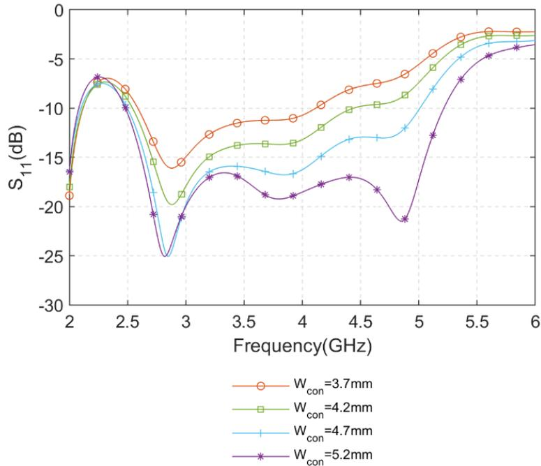
Fig. 4.15: Simulated  $S_{11}$  of the proposed CP Pseudo-ME dipole antenna with different  $W_{Con}$
