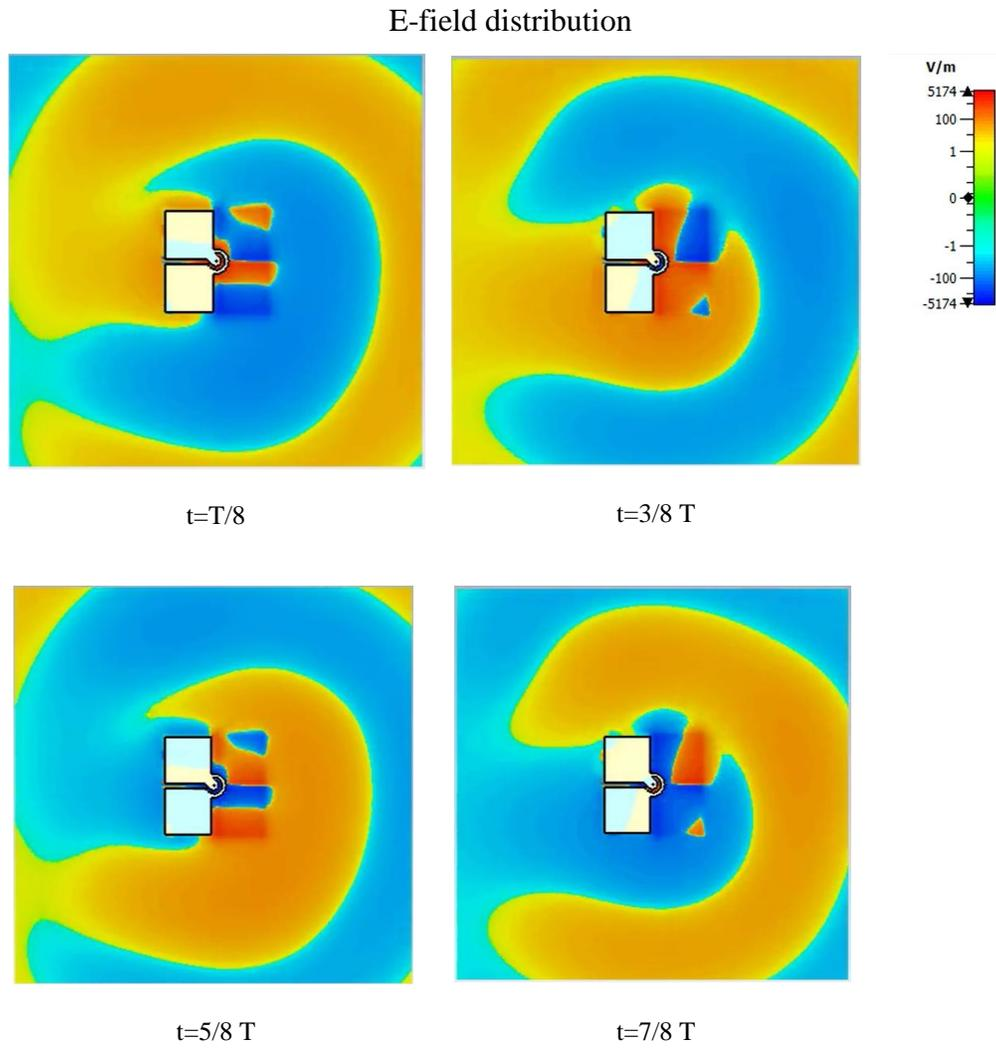
Fig. 4.7: E-field z-axis components distribution at different time
