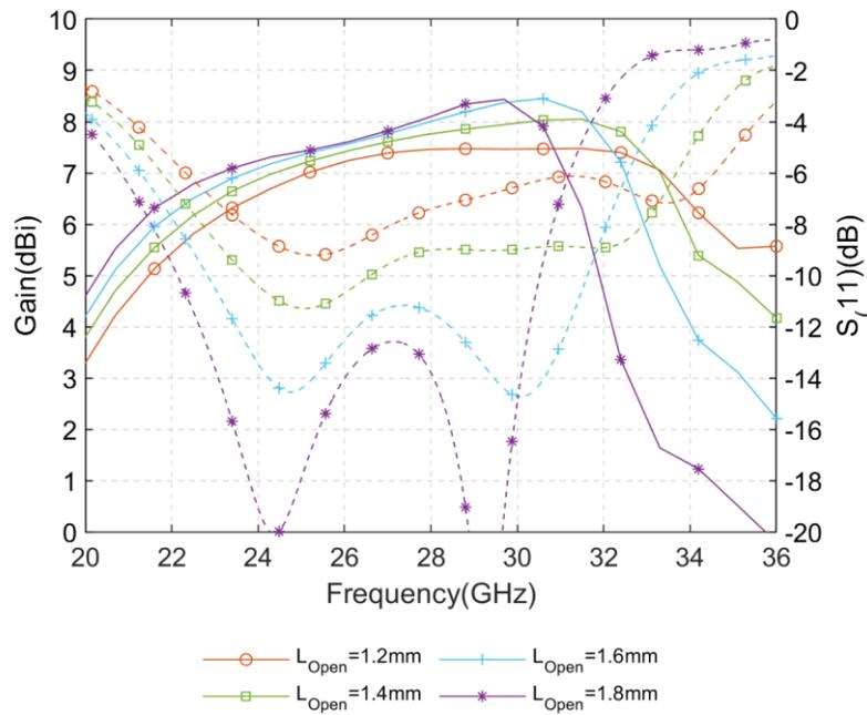
Fig. 5.27: Simulated  $S_{11}$  and gain of the mmW Pseudo-ME dipole antenna with different  $L_{Open}$
