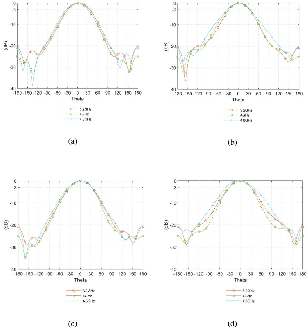
Fig. 4.38: Simulated radiation patterns at 3.2 GHz, 4 GHz, and 4.8 GHz when (a)  $\phi=0^\circ$ , (b)  $\phi=45^\circ$ , (c)  $\phi=90^\circ$ , (d)  $\phi=135^\circ$ .
