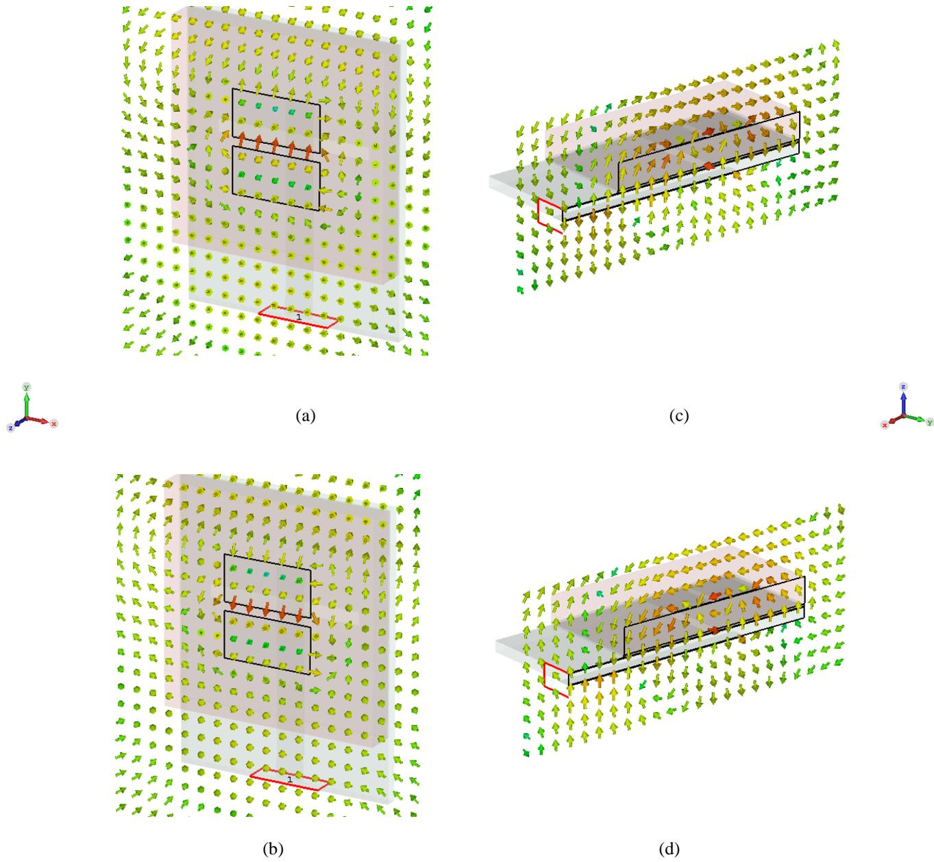
Fig. 5.5: E-field of the proposed antenna at center frequency 27.2 GHz (a)  $t = 0$ ; (b)  $t = T/2$  in  $xy$  plane; (c)  $t = T/4$ , (d)  $t = 3T/4$  in  $yz$ -plane
