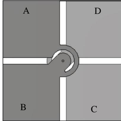
Fig. 4.9: Top view of left-hand polarization CP Pseudo-ME dipole antenna
