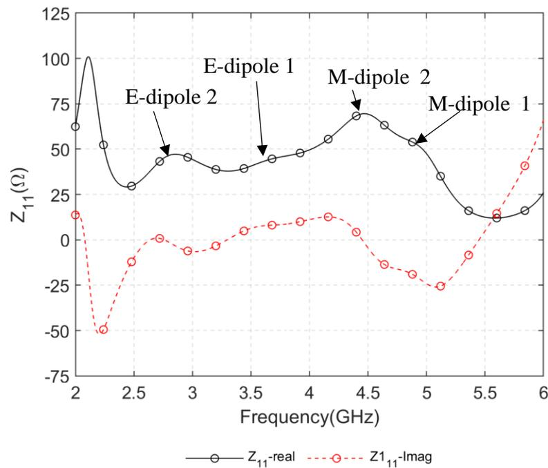
Fig. 4.34:  $Z_{11}$  of the CP Pseudo-ME dipole antennas under test
