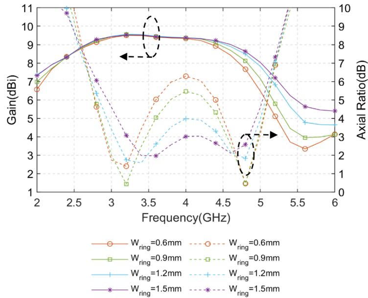
Fig. 4.20: Simulated gain and the axial ratio of the proposed CP Pseudo-ME dipole antenna with different  $W_{Ring}$
