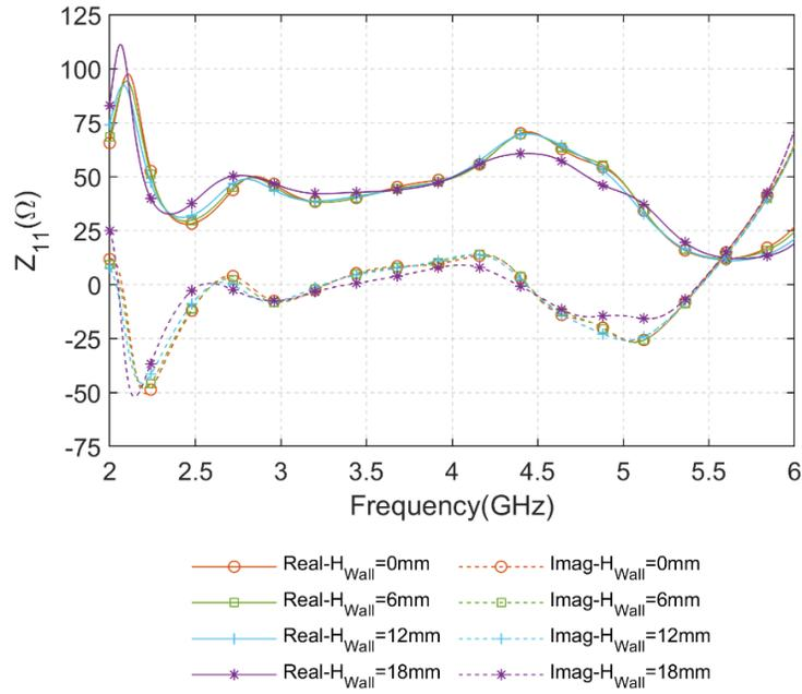
Fig. 4.45: Simulated  $Z_{11}$  of the proposed antenna with different  $H_{Wall}$
