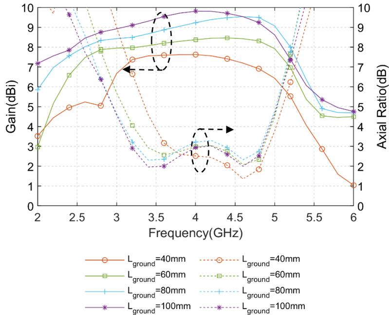
Fig. 4.29: Simulated gain and the axial ratio of the proposed CP Pseudo-ME dipole antenna with different  $L_{\text{Ground}}$
