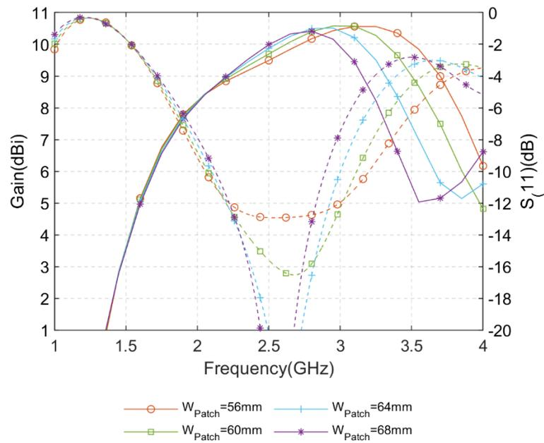
Fig. 3.7: Gain and  $S_{11}$  of the cavity-less Pseudo-ME dipole antenna at different patch width
