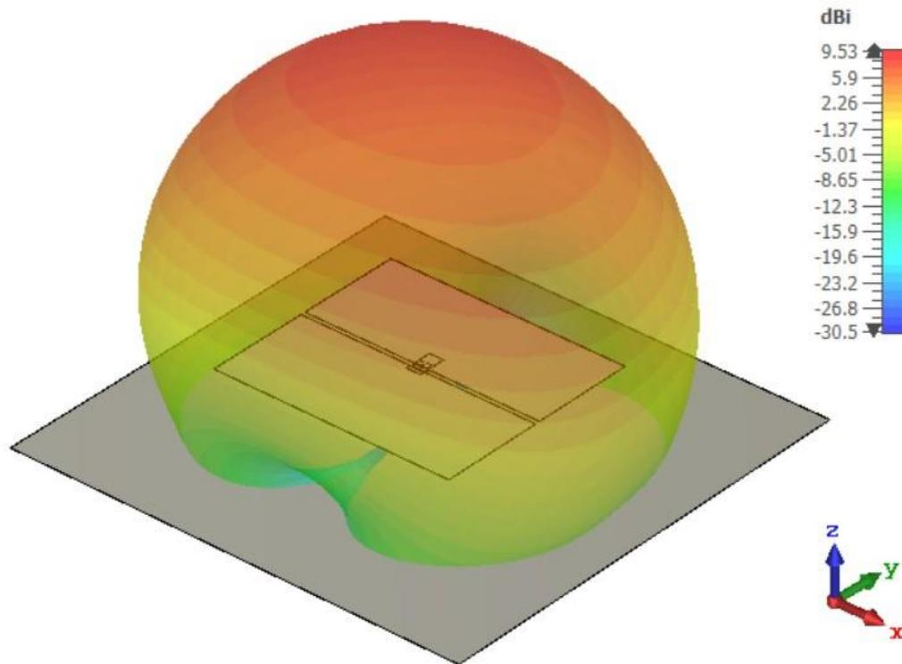
Fig. 3.18: Simulated radiation patterns of the proposed antenna in 3D
