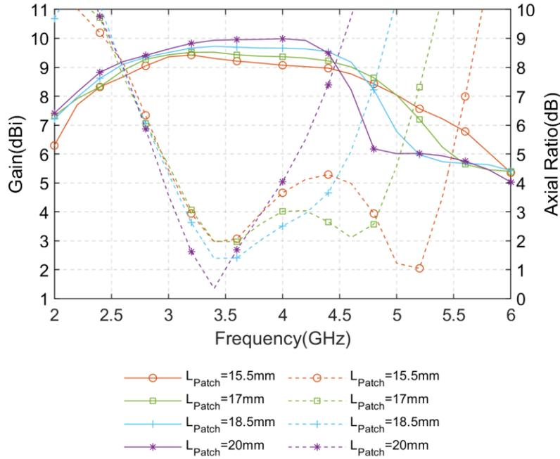
Fig. 4.14: Simulated gain and the axial ratio of the proposed CP Pseudo-ME dipole antenna with different  $L_{Patch}$
