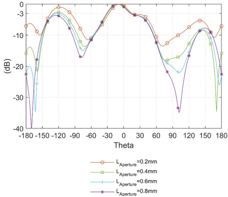
Fig. 5.21: E-plane radiation pattern of at 31.5 GHz with different  $L_{\text{Aperture}}$
