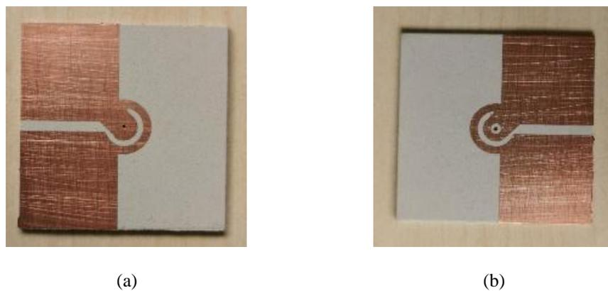
Fig. 4.32: (a) Top side of the radiating layer (b) the bottom side of the radiating layer of the fabricated radiating layer
