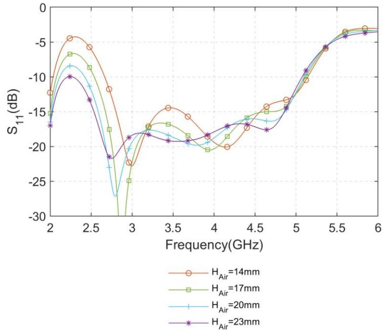
Fig. 4.24: Simulated  $S_{11}$  of the proposed CP Pseudo-ME dipole antenna with different  $H_{Air}$
