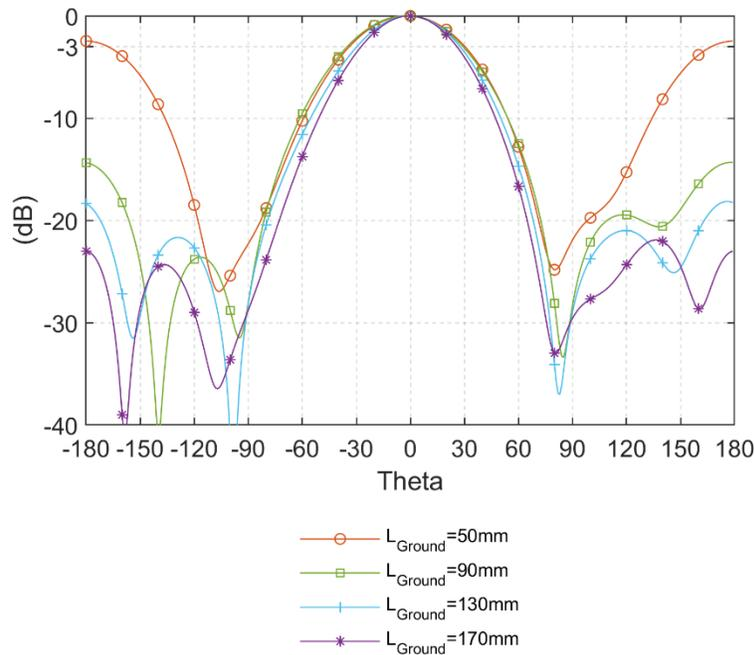
Fig. 3.12: E plane Radiation patterns of cavity-less Pseudo-ME dipole antenna with the different ground size ( $L_{\text{Ground}}$ )
