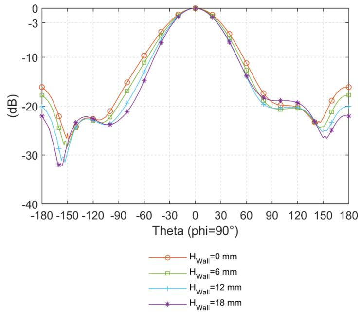
Fig. 4.49: Radiation pattern of the CP Pseudo-ME dipole antenna with different  $H_{Wall}$  when
