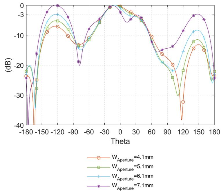
Fig. 5.26: E-plane radiation pattern of at 31.5 GHz with different  $W_{\text{Aperture}}$
