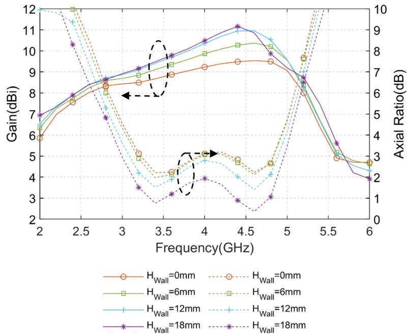
Fig. 4.46: Simulated gain and the axial ratio of the proposed antenna with different  $H_{Wall}$
