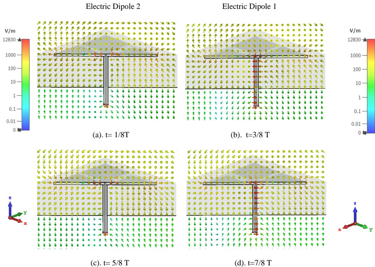
Fig. 4.4: The electric field of the two electric dipoles at different times.
