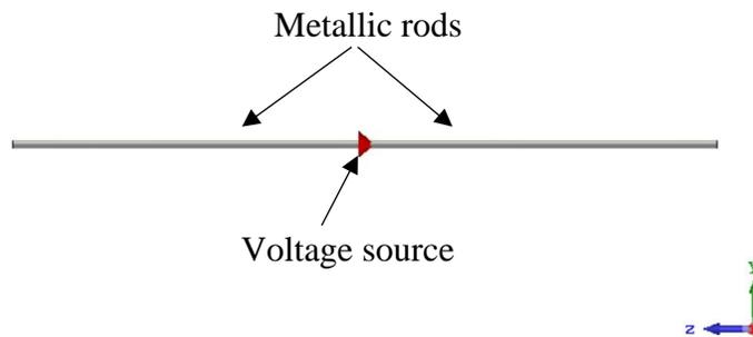
Fig. 2.7: The geometry of a half-wavelength dipole
