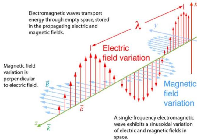
Fig. 2.1: Electromagnetic waves [1]
