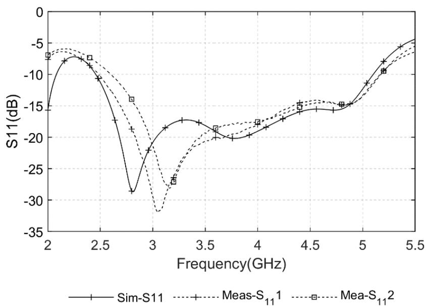
Fig. 4.33:  $S_{11}$  of the CP Pseudo-ME dipole antennas under test
