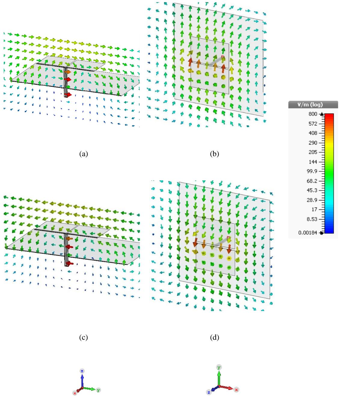
Fig. 3.2: E-field of electric dipole mode. yz plane cut (a).  $t = 0$ ; (b).  $t = T/2$ ; xy plane cut (c).  $t = T/2$ ; (d).  $t = T/2$
