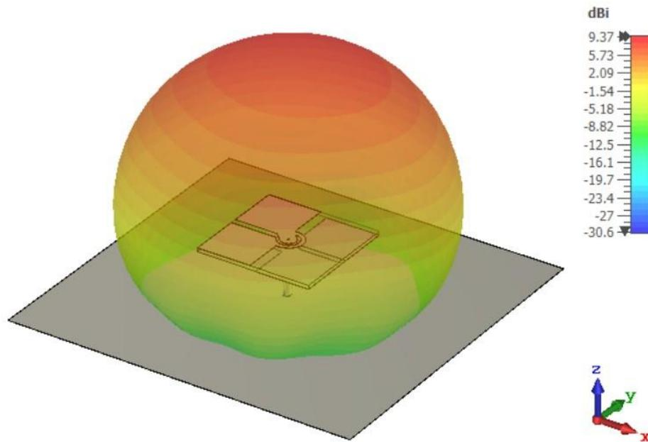
Fig. 4.37: Simulated radiation patterns at 4 GHz in 3D
