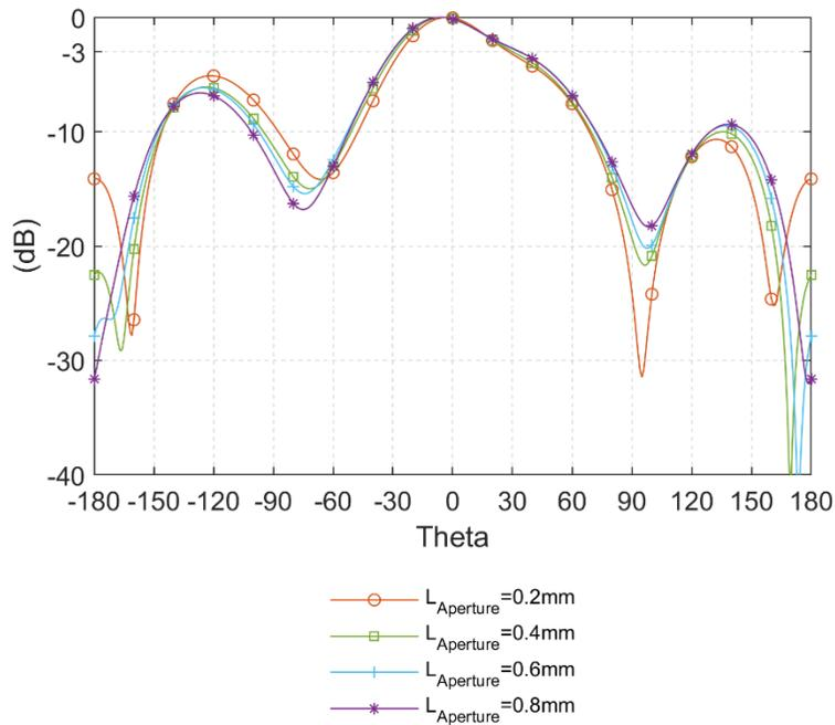
Fig. 5.20: E-plane radiation pattern at 27.5 GHz with different  $L_{\text{Aperture}}$
