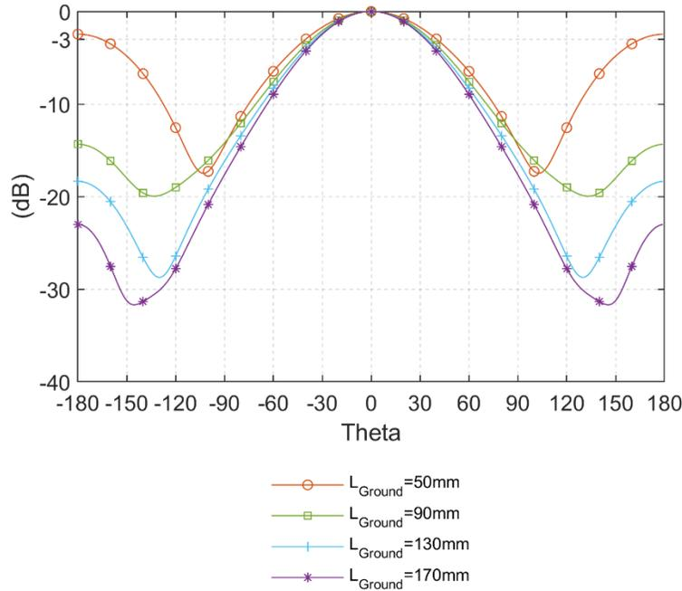
Fig. 3.13: H plane radiation patterns of cavity-less Pseudo-ME dipole antenna with the different ground size ( $L_{Ground}$ )
