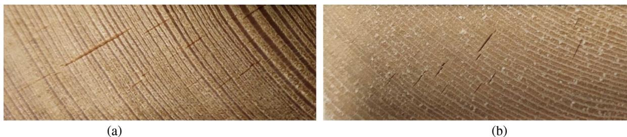
**Figure 3:** End surfaces of considered species after exposure to freeze-thaw cycles (a) *Larix gmelinii* specimens (b) *Pinus sylvestris* specimens
