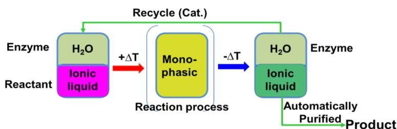
**Figure 6.** Functional solvents: Automatic reaction/separation replacing respective equipment
