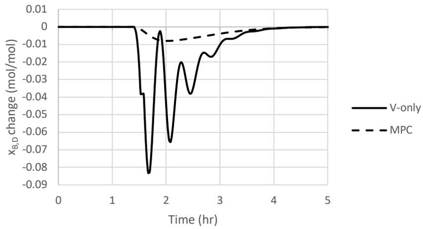
Figure 16: Difference in bottom product purity response to feed flow rate disturbance using conventional V-only control (solid line) and linear MPC (dashed line) for Case study 1. Disturbance introduced at  $t=1.4$  hrs.
