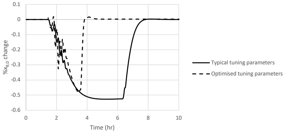
Figure 14: Bottom product purity response to feed flow rate disturbance (Case study 1, LV control) for typical and optimal tuning parameters. Disturbance introduced at  $t=1.4$  hrs. Optimised tuning parameters are shown in Table 5.
