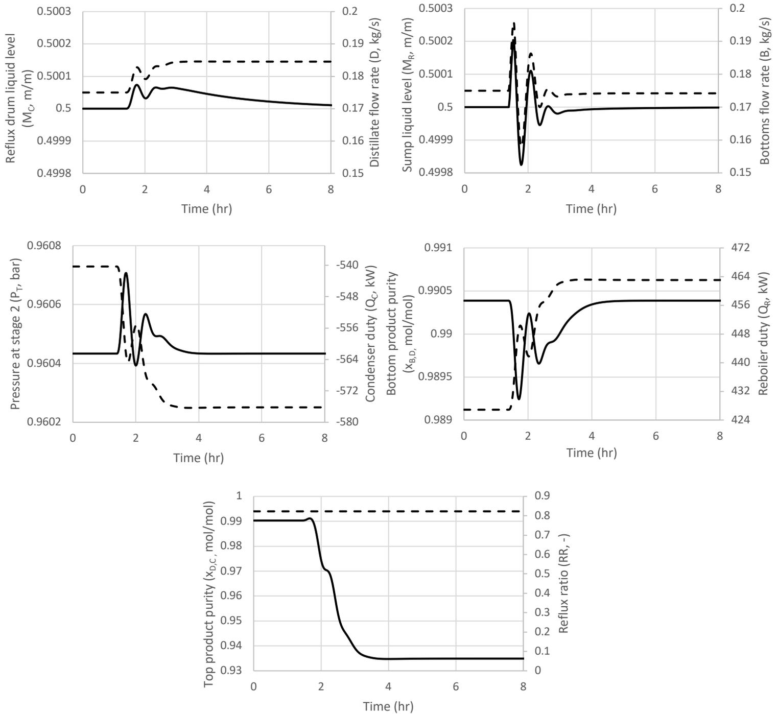
Figure 3: Closed-loop responses for feed B flow rate disturbance (5% increase). Disturbance introduced at  $t=1.4$  hrs. Left axis is controlled variable (solid line) and right axis is manipulated variable (dashed line). (Case study 2, V-only control).
