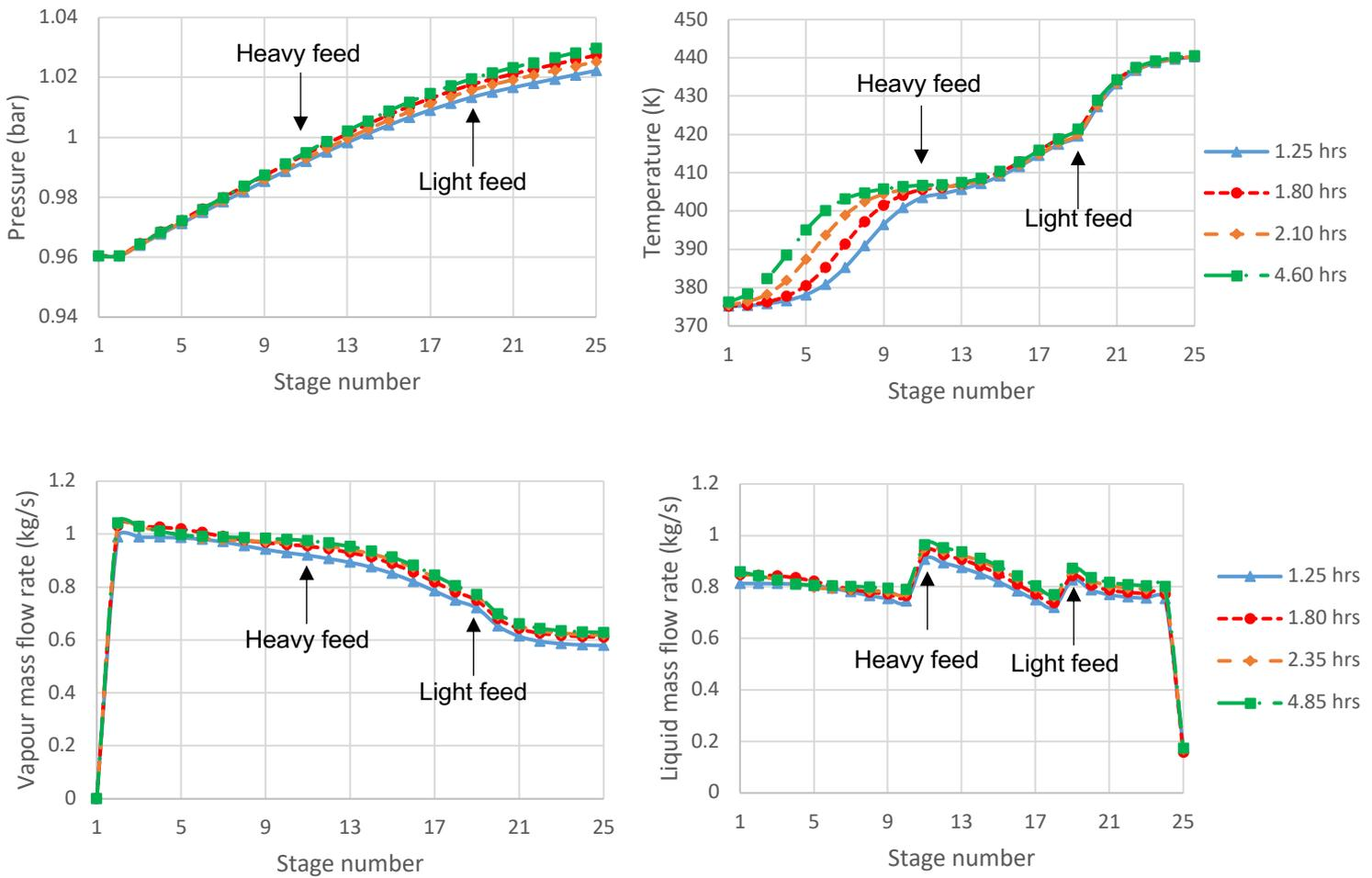
Figure 4: Pressure (top, left), temperature (top, right), vapour mass flow rate (bottom, left) and liquid mass flow rate (bottom, right) change due to the introduction of feed B flow rate disturbance (5% increase). Disturbance introduced at  $t=1.4$  hrs. (Case study 2, V-only control).
