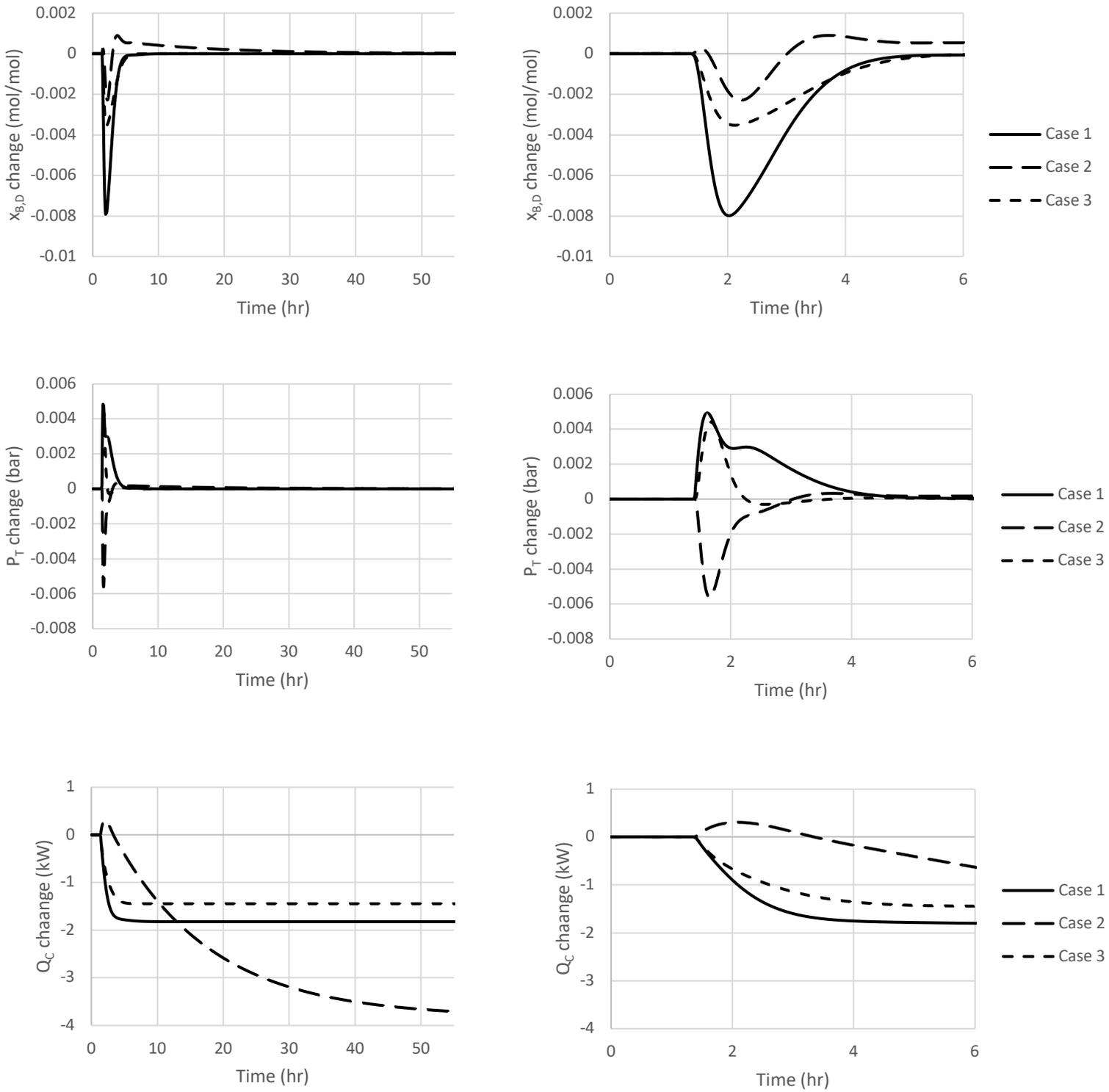
Figure 18: Control performance of MPC for all case studies towards feed B flow rate disturbance. Bottom product purity, pressure and condenser duty are presented from top to bottom, respectively. Left figures show full time scale whilst figures on the right focus on initial responses. Disturbance introduced at  $t=1.4$  hrs.
