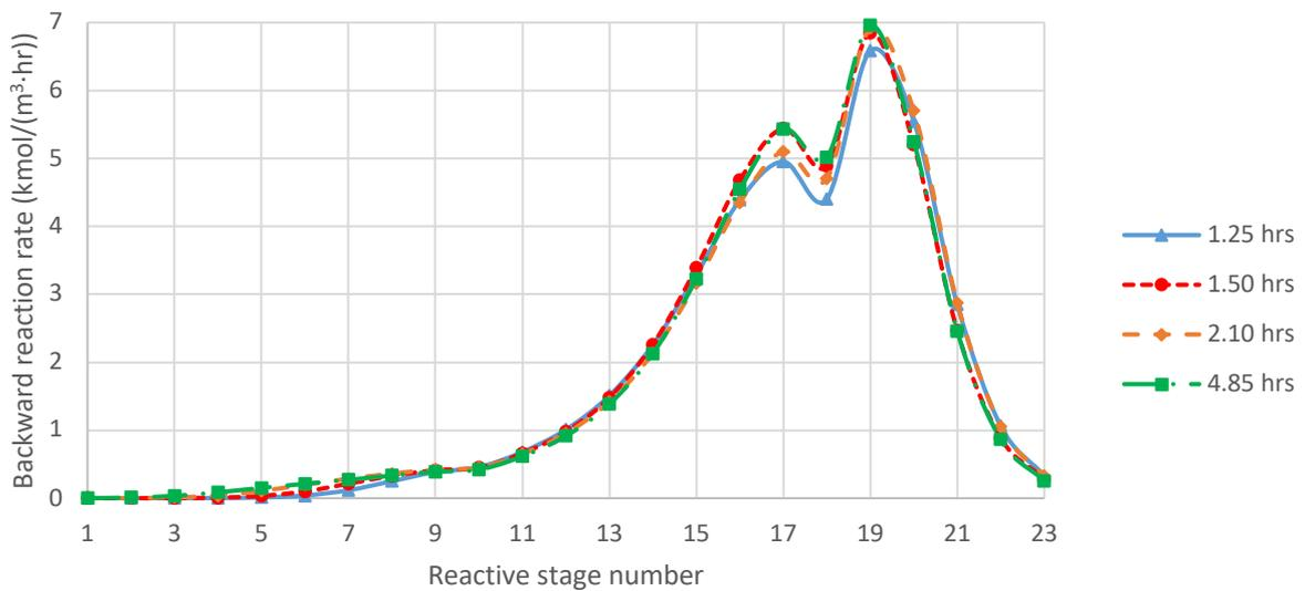
Figure 5: Reaction rate (forward-top and backward-bottom) change due to the introduction of feed B flow rate disturbance (5% increase). Disturbance introduced at  $t=1.4$  hrs. Stages 1 (condenser) and 25 (reboiler) are not considered reactive, therefore reactive stages only are shown. (Case study 2, V-only control).
