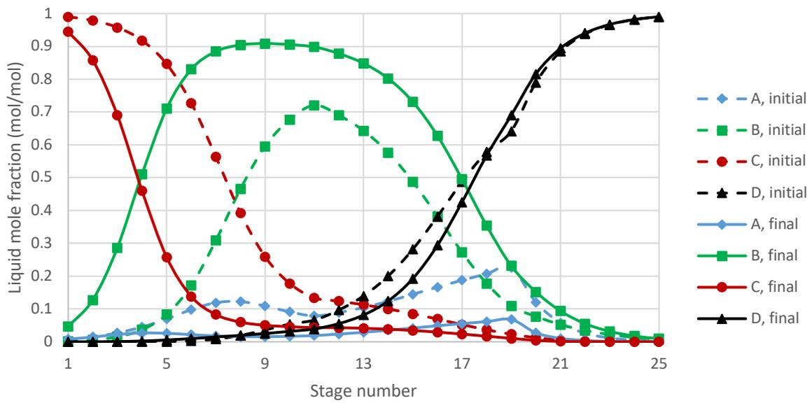
Figure 10: Composition profiles change due to feed B flow rate disturbance (5% increase).
