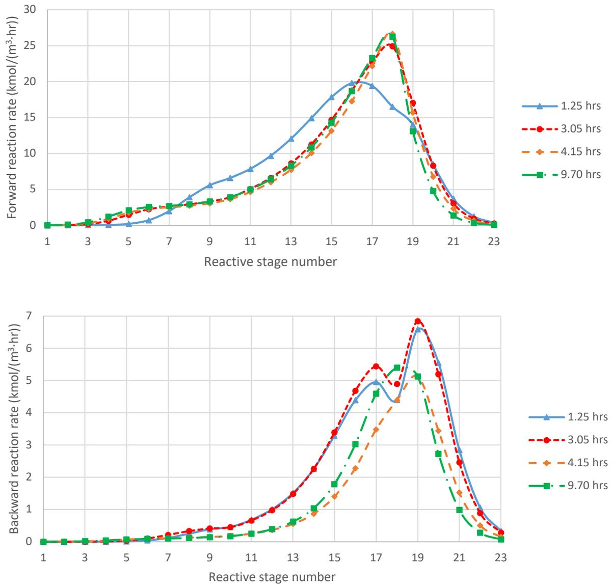
Figure 9: Reaction rate (forward-top and backward-bottom) change due to the introduction of feed B flow rate disturbance (5% increase). Disturbance introduced at  $t=1.4$  hrs. Stages 1 (condenser) and 25 (reboiler) are not considered reactive, therefore reactive stages only are shown. (Case study 2, LV control).
