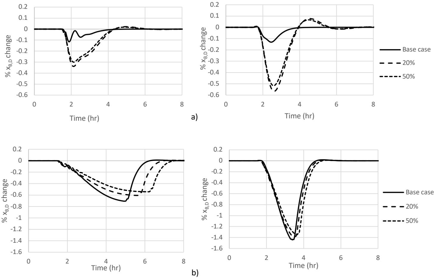
Figure 13: Bottom product purity response to feed flow rate (left) and feed composition (right) disturbance for increased tray liquid holdup. Disturbance introduced at  $t=1.4$  hrs. (Case study 2, V-only (a) and LV (b) control).
