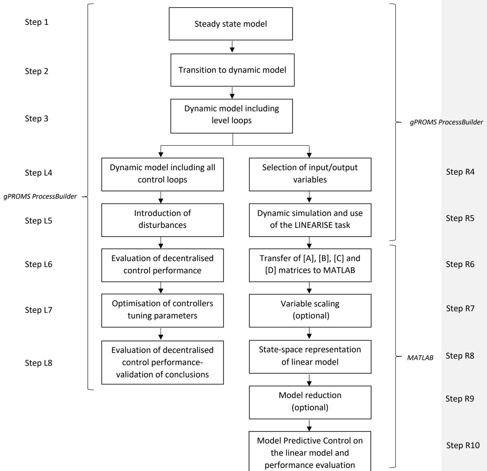
Figure 1: Methodology proposed in this work for the evaluation of controllability using conventional and advanced control strategies. Left: evaluation of conventional control schemes within gPROMS ProcessBuilder, Right: evaluation of Model Predictive Control on a linearised model using both gPROMS ProcessBuilder and MATLAB. The methodology should be repeated several times based on the purpose of the investigation as explained in section 2.
