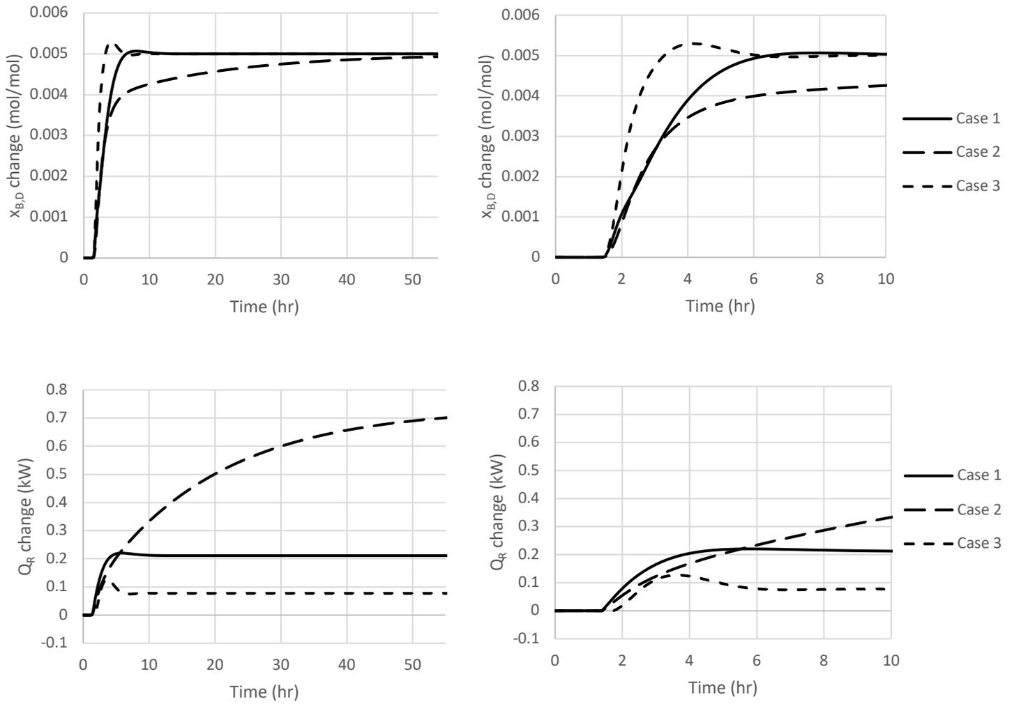
Figure 17: Control performance of MPC for all case studies towards bottom product purity set point change. Bottom product purity response and reboiler duty are presented from top to bottom, respectively. Left figures show full time scale whilst figures on the right focus on initial responses. Disturbance introduced at  $t=1.4$  hrs.
