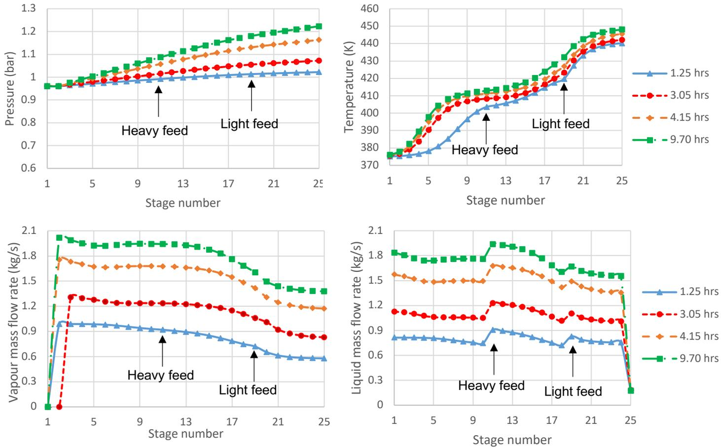
Figure 8: Pressure (top, left), temperature (top, right), vapour mass flow rate (bottom, left) and liquid mass flow rate (bottom, right) change due to the introduction of feed B flow rate disturbance (5% increase). Disturbance introduced at  $t=1.4$  hrs. (Case study 2, LV control).
