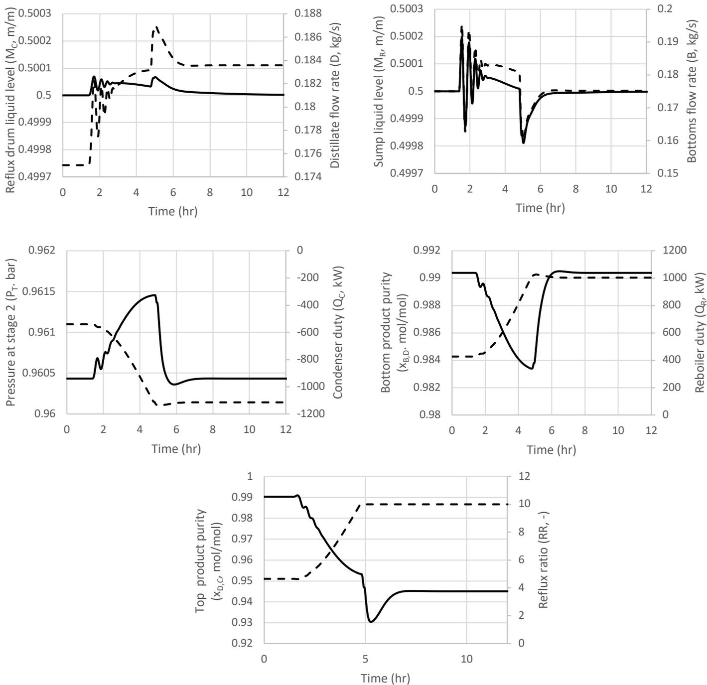
Figure 7: Closed-loop responses for feed B flow rate disturbance (5% increase). Disturbance introduced at t=1.4 hrs. Left axis is controlled variable (solid line) and right axis is manipulated variable (dashed line). (Case study 2, LV control).
