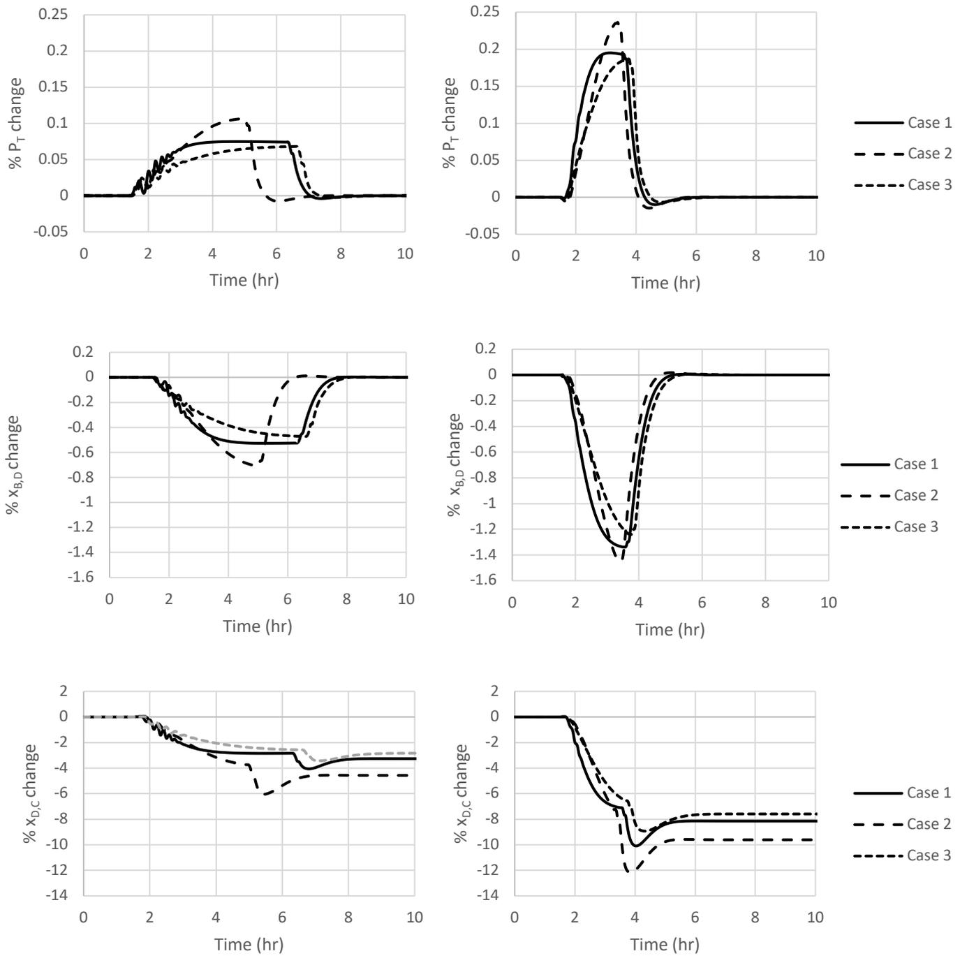
Figure 11: Response to feed flow rate disturbance (5% Feed B increase) (left) and feed composition disturbance (5% Feed B increase and 5% Feed A decrease) (right) for all case studies. Disturbance introduced at t=1.4 hrs. Top: pressure; Middle: Bottom product purity; Bottom: Top product purity. (LV control).
