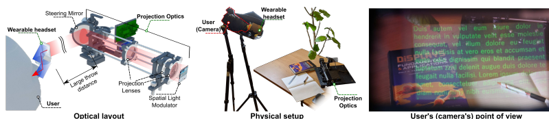
Fig. 1. Beaming Displays. Left: Our new optical layout decomposes a near-eye display design into two parts, an all passive light-weight wearable headset, and a remotely located projector, this decomposition effectively avoids trade-offs between ergonomics, computational and power requirements. Middle: We build a physical setup to demonstrate the possibilities with our optical layout. Right: We show experimentally that our design supports resolutions matching a consumer level near-eye display.
