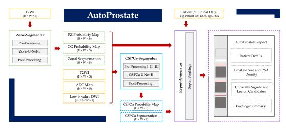
**Figure 1.** AutoProstate framework diagram. AutoProstate consists of three modules: Zone-Segmenter (green), CSPCa-Segmenter (blue), and Report-Generator (purple); solid boxes correspond to module computations, while dashed boxes correspond to module outputs. Yellow boxes indicate AutoProstate inputs from external sources.
