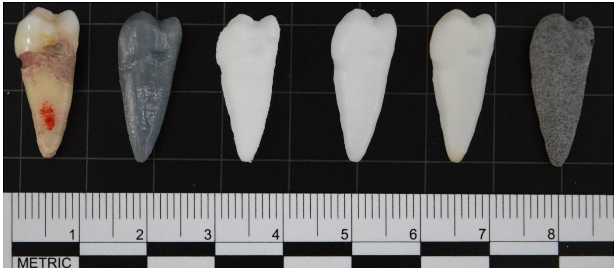
Figure 1. 3D printed teeth and original tooth from left to right: Natural tooth, FDM printed tooth, SLS printed tooth, DLP printed tooth, SLA printed tooth and MJF printed tooth.
