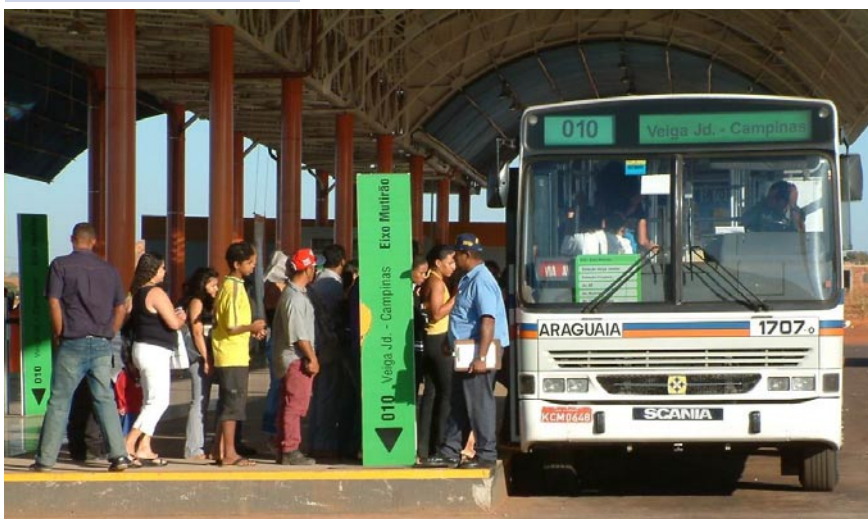
Fig. 31 ▼ On-board fare collection creates delays and problems in Goiania, Brazil. Lloyd Wright
