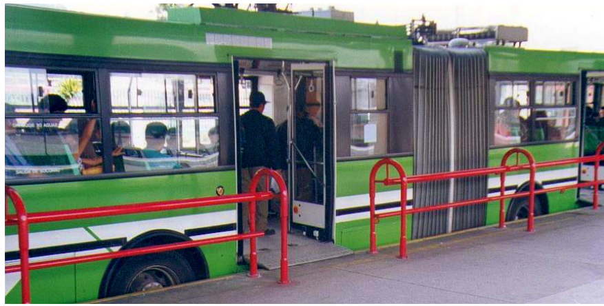
Fig. 25 ▲ Flip-down entry ramps in Quito, Ecuador. Lloyd Wright
