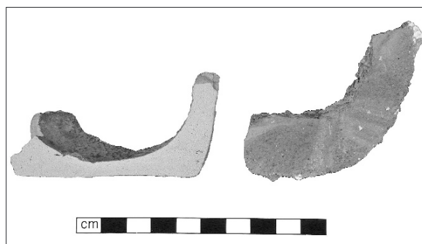
Fig. 7: Photograph of a cross section through the bottom part of a crucible from Akhsiket (left) and Konasamudram (right), for comparison. Note the different colour and thickness of the ceramic. Photo: S. Laidlaw, IoA, London.
