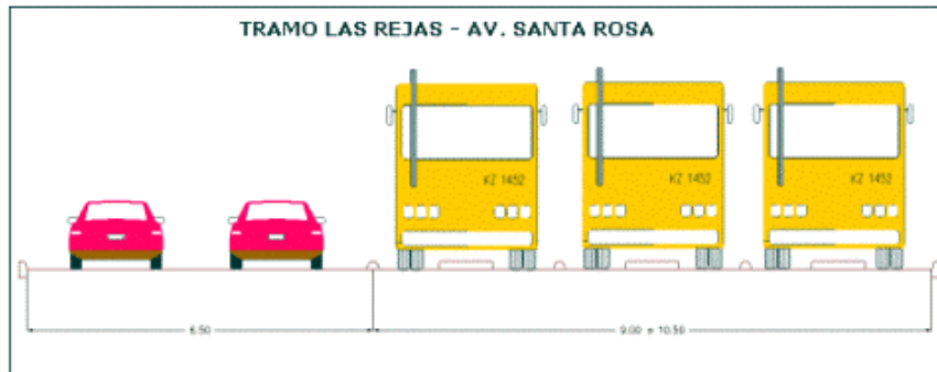
Fig. 7: Bus-lane scheme in Alameda, Santiago (right hand driving)
