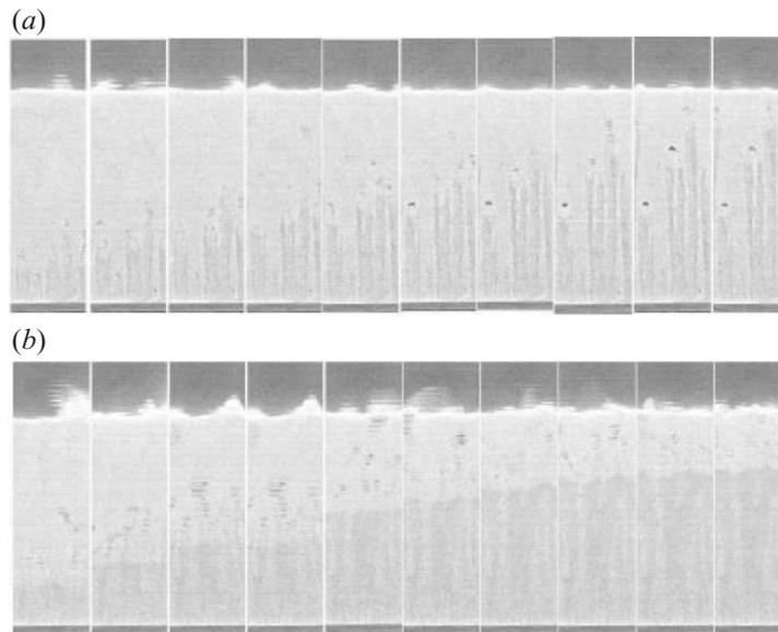
FIGURE 1. Time sequence showing the formation of segregation patterns by gas flowing through an initially homogeneous mixture of particles with equal proportions of 45–90  $\mu\text{m}$  and 250–425  $\mu\text{m}$  particles. The initial bed height is 12.0 cm. In (a) the gas flow rate is 1.9  $\text{cm s}^{-1}$  and the time difference between each image is 1.0 s, and in (b) the gas flow rate is 3.88  $\text{cm s}^{-1}$  and the time difference is 2.0 s.
