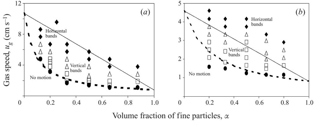
FIGURE 3. Phase diagrams for the mixtures of particles based on experimental observations. The different symbols correspond to the different structures seen: incipient motion ( $\bullet$ ); vertical bands ( $\square$ ); partial segregation ( $\triangle$ ); horizontal banding ( $\blacklozenge$ ). (a) A mixture of 45–90  $\mu\text{m}$  particles and 250–425  $\mu\text{m}$  particles, and (b) a mixture of 45–90  $\mu\text{m}$  particles and 190–212  $\mu\text{m}$  particles.
