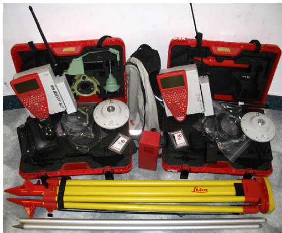
Figure 2: Dual Leica System SR530 geodetic GPS receivers
