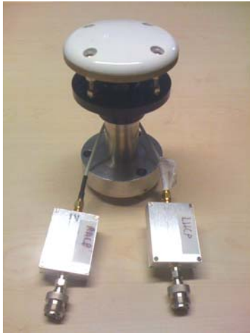
Figure 1: Antcom 3G1215RL-P-XS-1 dual-polarization antenna, mounting and amplifiers.
